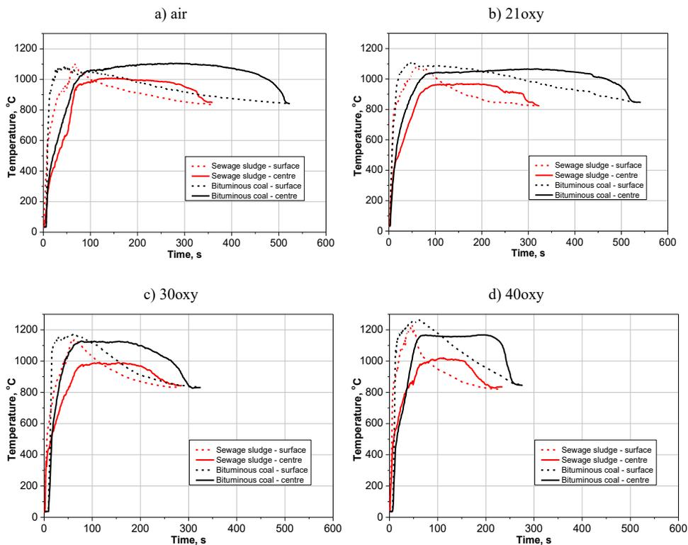
Fig. 6. Temperature profiles for sewage sludge and bituminous coal burned at 850°C in various atmospheres.
