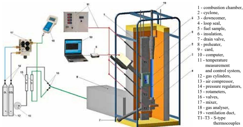
Fig. 1. Schematic diagram of the experimental apparatus for oxy-CFB combustion
