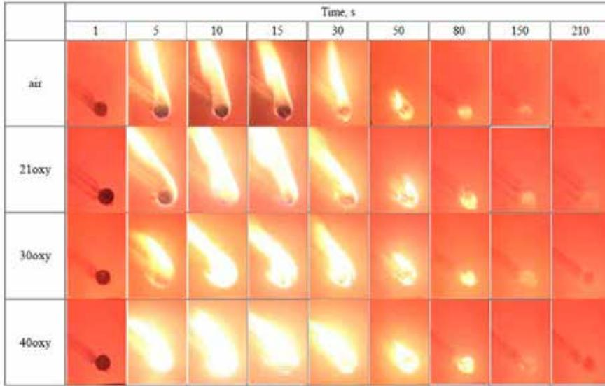
Fig. 2. Combustion of sewage sludge in air and O<sub>2</sub>/CO<sub>2</sub> mixtures at 850°C.
