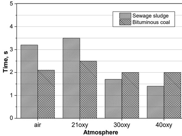
Fig. 3. Average ignition time for sewage sludge and bituminous coal burned in various atmospheres at 850 °C.
