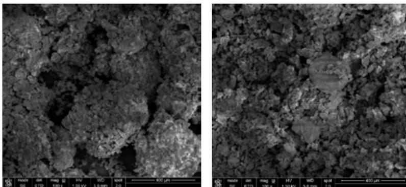
Fig. 7. SEM images of sewage sludge ashes obtained during combustion (air atmosphere) 21%O<sub>2</sub>/79% N<sub>2</sub>.
