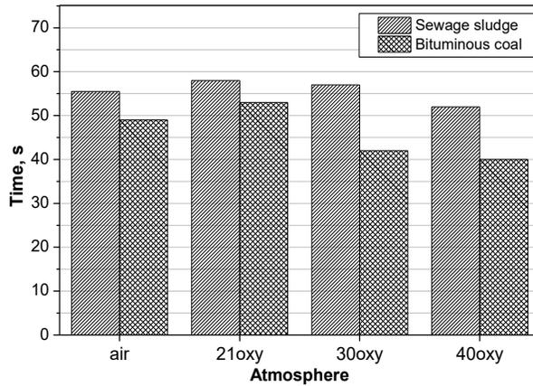
Fig. 4. Average devolatilization time for sewage sludge and bituminous coal burned in various atmospheres at 850 °C.
