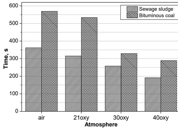
Fig. 5. Average total combustion time for sewage sludge and bituminous coal burned in various atmospheres at 850 °C.
