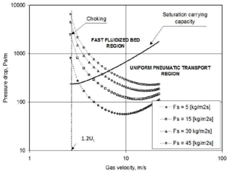
Fig. 2. Phase diagram of solid – gas flow (calculated for tube diameter –  $0.059mm$ , particle diameter –  $0.5mm$ , solid density-  $1250 kg/m^3$ , air at ambient conditions).
