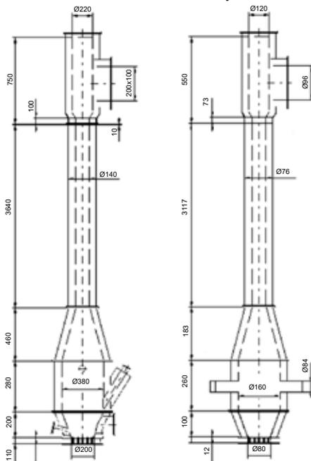
Fig. 1. Schematic diagram of CFB gasification reactors. From left – ambient pressure reactor, from right – pressurized reactor.
