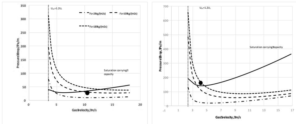
Fig. 3 Comparison of pressure drop for  $P=0.1MPa$  and  $P=0.5MPa$ . (Black dot – operating point)
