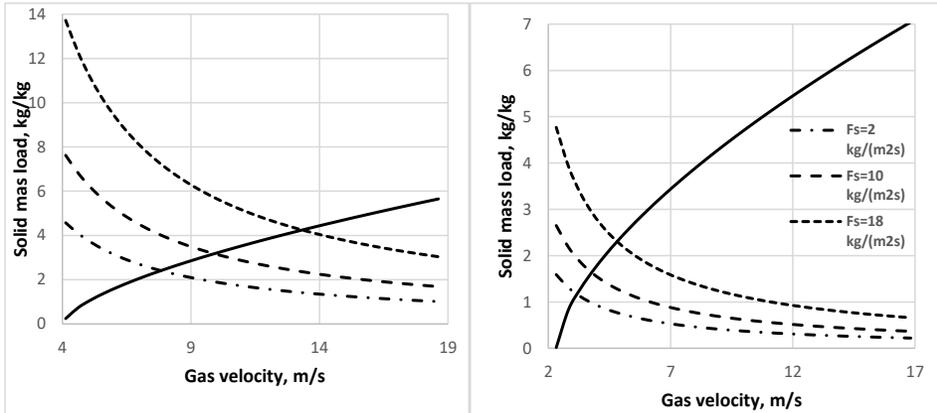
Fig. 4 Critical loading of solids for P=0.1MPa and P=0.5MPa.
