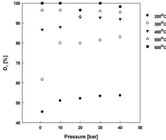
Fig. 3. Effect of drying ratio on operation pressure
