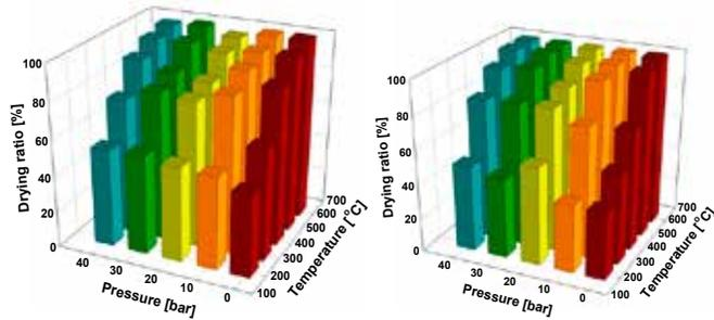
Fig. 4. Effect of drying ratio on operation temperature and pressure
