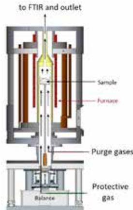
Figure 1: Cross sectional view of the TGA analyzer.
