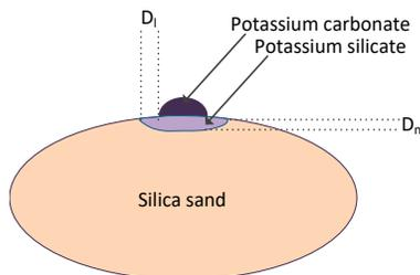
Figure 6: Schematic representation of initial stage of reaction between  $K_2CO_3$  and silica sand
