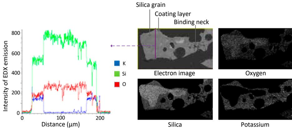
Figure 5: SEM-EDX analysis of imbedded samples.  $\text{SiO}_2:\text{K}_2\text{CO}_3$  ratio = 3:100;  $T= 850\text{ }^\circ\text{C}$ ; pure  $\text{N}_2$  atmosphere; well mixed sample; powder form of  $\text{K}_2\text{CO}_3$ ; isothermal reaction time 4h.
