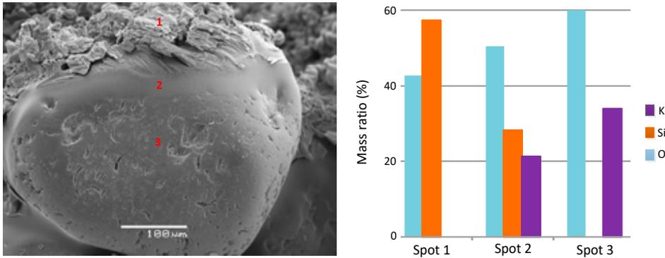
Figure 4: SEM-EDX analysis of a representative reaction product:  $\text{SiO}_2:\text{K}_2\text{CO}_3$  ratio = 3:100;  $T= 800\text{ }^\circ\text{C}$ ; pure  $\text{CO}_2$  atmosphere; segregated mixture; powder form of  $\text{K}_2\text{CO}_3$ ; isothermal reaction time 4h.
