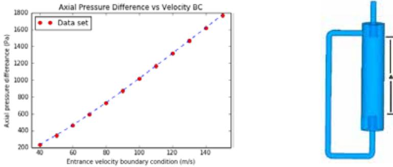
Figure 8: Effect of Entrance Condition on Axial Pressure Difference
