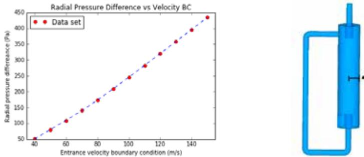
Figure 6: Effect of Entrance condition on Radial pressure difference
