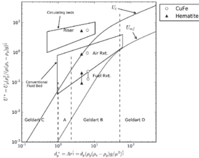
Fig. 3. Flow regime map showing where the air reactor, fuel reactor, and riser operate in the CLR. Map based on plot from Grace (1986).
