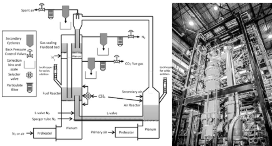
Fig. 2. Chemical looping reactor at NETL
