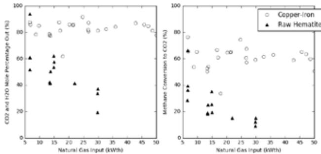
Fig. 6. (a) Species purities for CO<sub>2</sub> and steam (minus the nitrogen diluent) and (b) Methane conversion to CO<sub>2</sub> as a function of natural gas input.
