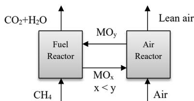
Fig. 1. Chemical looping combustion with natural gas as the fuel.
