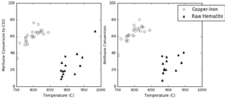
Fig. 4. Effect of temperature on the conversion of natural gas in the fuel reactor.
