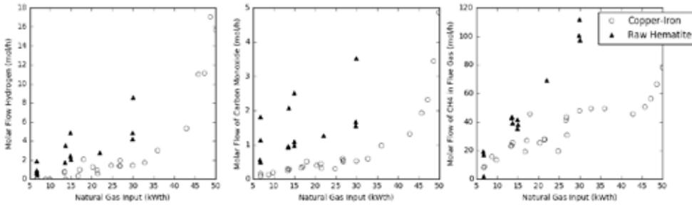
Fig. 5. Molar flow rates of product gases for each trial for the raw hematite and synthetic carrier.
