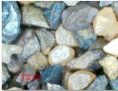
Fig. 2. Microscopic photograph of ilmenite - research material used in the study
