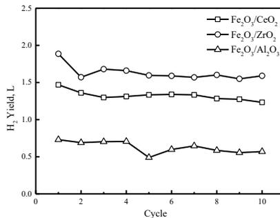
Fig. 2. Effect of cycle number on H<sub>2</sub> yield for oxygen carriers with different supports at 850°C
