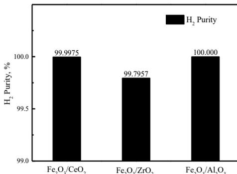
Fig. 3. Effect of different supports on H<sub>2</sub> purity at 850°C
