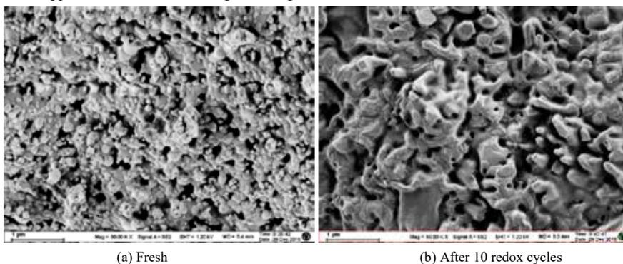
Fig.5. SEM images of the oxygen carrier  $\text{Fe}_2\text{O}_3/\text{CeO}_2$
