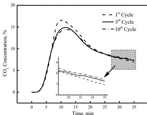
Fig. 4.  $\text{CO}_2$  concentration in reduction stage for  $\text{Fe}_2\text{O}_3/\text{CeO}_2$  in the 1<sup>st</sup>, 3<sup>rd</sup> and 10<sup>th</sup> cycles at 850°C
