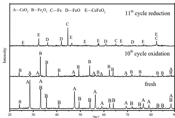
Fig.6. XRD patterns of the oxygen carrier  $\text{Fe}_2\text{O}_3/\text{CeO}_2$
