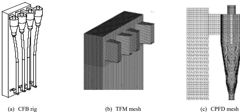
Fig. 1. CPFD geometry and CFD mesh
