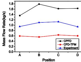
Fig. 9 Solid mass flow rate through the four cyclones
