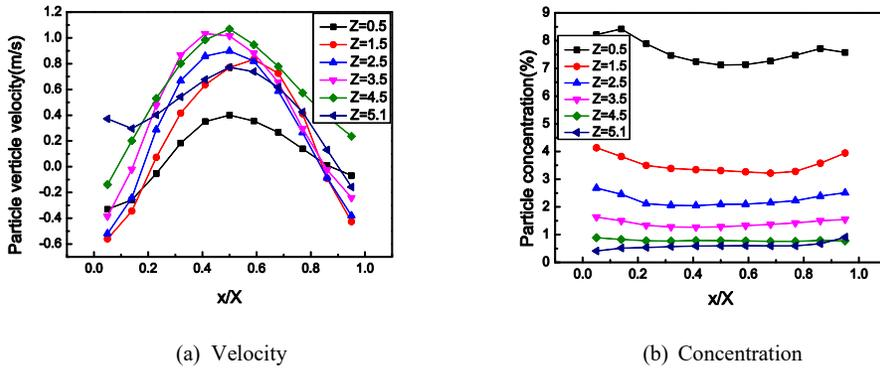
Fig. 8 particle velocity and concentration along the height of the riser
