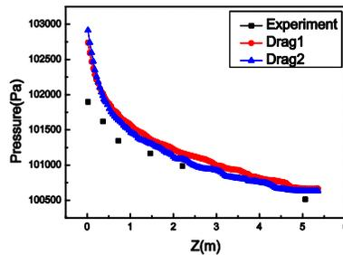
Fig. 3. Comparison between CPFD simulation and measurements
