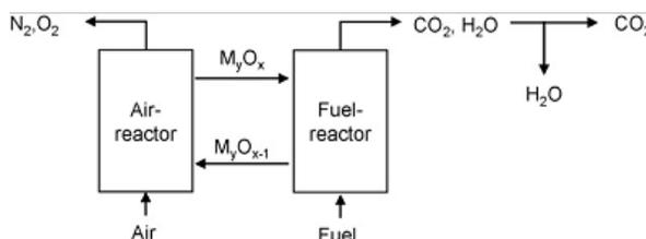
Fig. 1. Reactor scheme of the CLC process.
