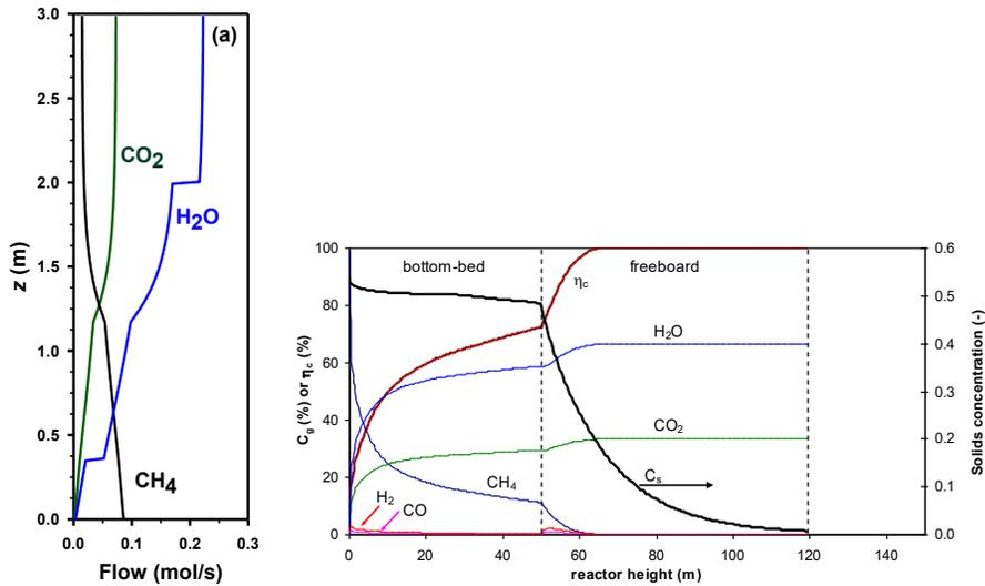
Fig. 2. Longitudinal profiles of gas and solids concentration in the fuel-reactor. (a) CFB fuel reactor model (b) BFB fuel reactor model.
