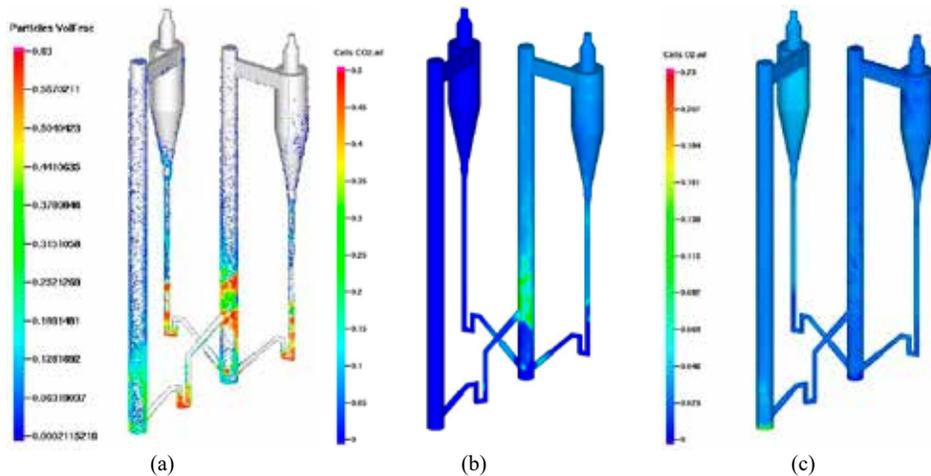
Fig. 8. Simulation of performance of CLOU PDU when processing coal. Figures show (a) particle volume fraction; (b) CO<sub>2</sub> concentration and (c) O<sub>2</sub> concentration. The air reactor is on the left, fuel reactor is on the right. Coal is fed into the bottom of the fuel reactor. Bed mass: 155 kg. Air reactor flow: 256 kg/h. Fuel reactor (steam) flow: 154 kg/h. T: 900°C.
