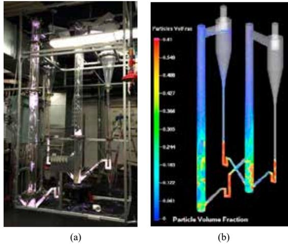
Fig. 3. (a): Cold flow model of the 200 kW PDU and (b) Barracuda simulation of the cold flow model showing particle volume fraction.
