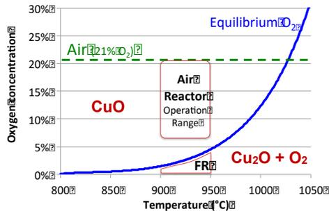
Fig. 1.  $\text{CuO}/\text{Cu}_2\text{O}$  equilibrium diagram showing the range of operating conditions for CLOU air and fuel reactors.
