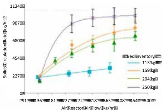
Fig. 7. Ilmenite circulation rates in PDU, measured at approx. 600°C.
