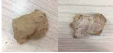
Fig. 8. The ash deposit sample of the economizer heating surface.
