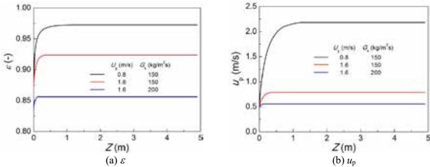
Fig. 3 Effects of operation conditions on the axial profiles of  $\epsilon$  and  $u_p$
