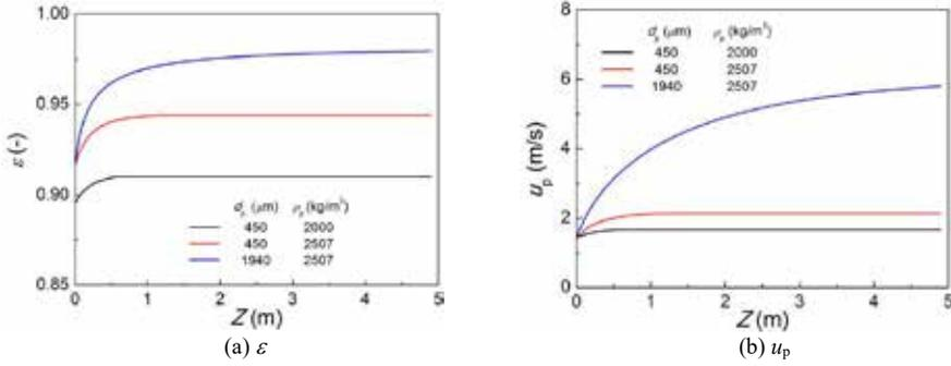
Fig. 4 Effects of particle properties on the axial profiles of  $\varepsilon$  and  $u_p$
