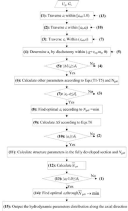
Fig. 2 Numerical scheme for solving the EMMS-based counter-current gas-solid downer model
