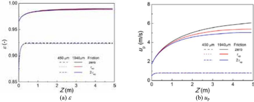
Fig. 5 Effect of wall friction on the axial profiles of  $\varepsilon$  and  $u_p$
