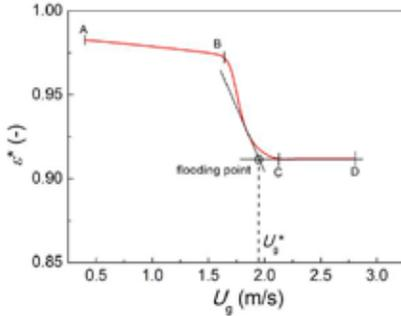
Fig. 6 Determination of  $U_g^*$
