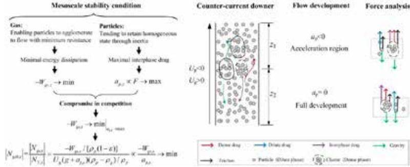
Fig. 1 Physical basis of the EMMS-based model for counter-current gas-solid downward flow
