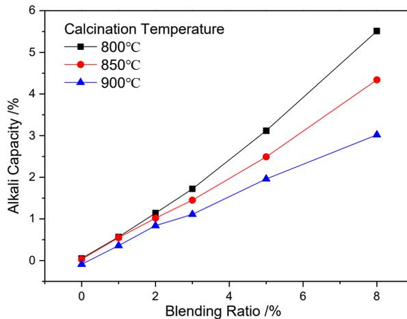
Fig. 6. Influence of blending ratio on alkali capacity of bed material.
