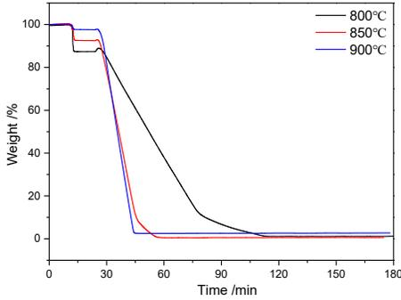
Fig.3. Weight loss curve of NaCl.
