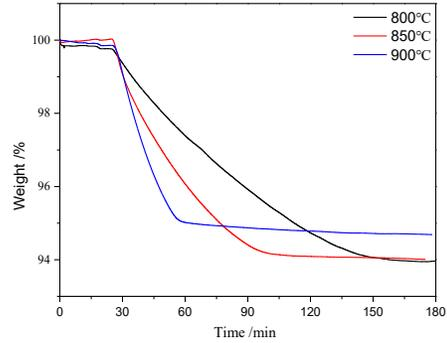
Fig.4. Weight loss curve of bed material.
