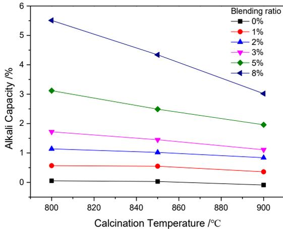
Fig. 5. Influence of calcination temperature on alkali capacity of bed material.
