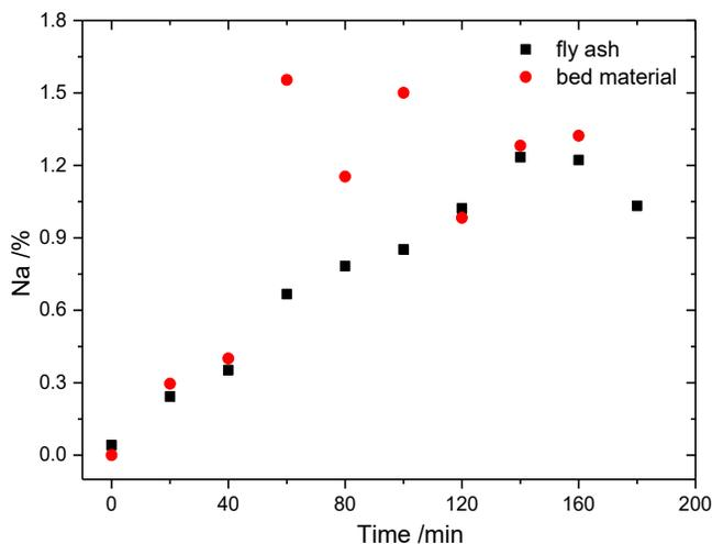
Fig. 8. Chang of sodium content in fly ash and bed material over time.
