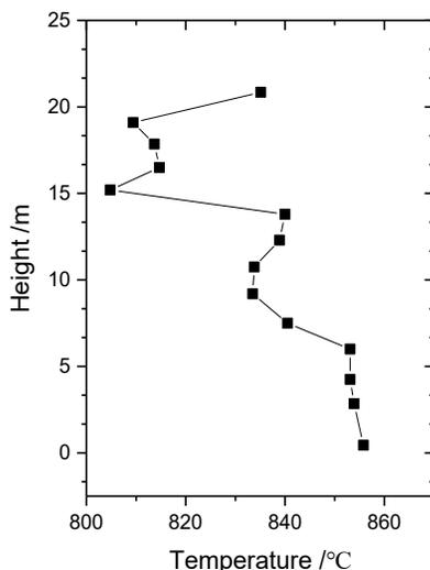
Fig.8. Temperature distribution along the furnace.
