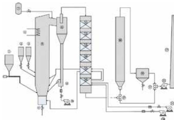
1.Coal bunker 2.Limestone bunker 3.Sand bunker 4.Water-cooled tubes 5.Furnace 6.Slagging pipe 7.Ammonia 8.Separator 9.Loop seal 10.Material-returning air fan 11-12.High temperature economizer 13-14.Low temperature economizer 15-16.Air pre-heater 17.Valve 18.Half dry desulfurization 19.Precipitator 20.Primary air fan 21.Secondary air fan 22.Induced draft fan 23.Chimney
