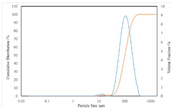
Fig.2. Particle size distribution of bed material.
