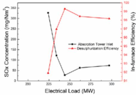
Fig. 4 Desulphurization efficiency by limestone particle injection into the furnace at different load
