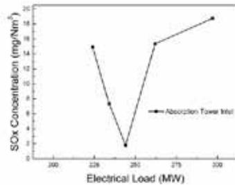
Fig. 5 SO<sub>2</sub> emission at different load
