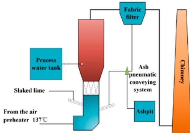
**Fig. 2 System diagram of circulating fluidized bed flue gas desulphurization**
