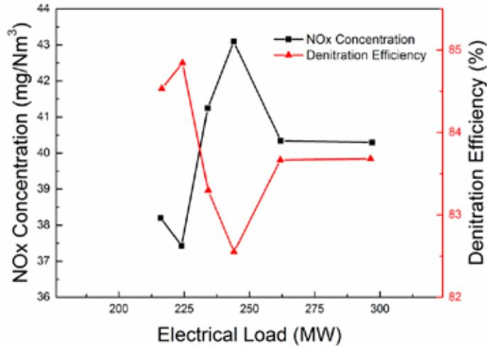
Fig. 6 NO<sub>x</sub> emission at different load
