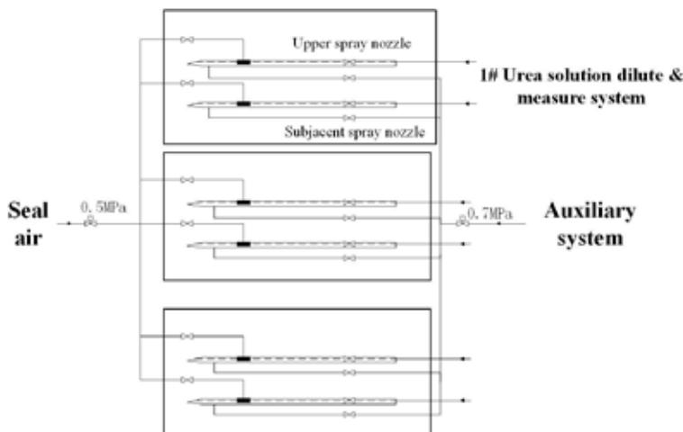
Fig. 3 System diagram of SNCR by urea solution
