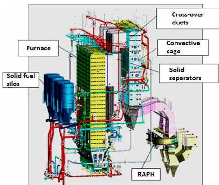
Fig.1 – Sketch of the Novocherkassk TPP unit#9 CFB boiler (FW data)
