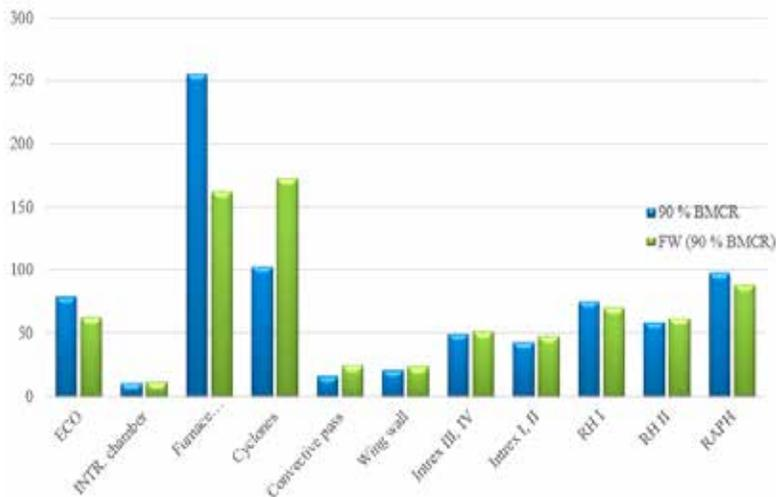
Fig. 6. Elementwise heat duty comparison at 90% BMCR
