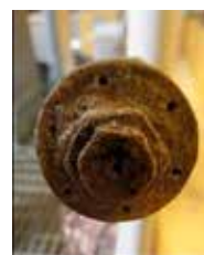
Fig 2. Rear end of lance and tip of a nozzle for injection of ammonium sulphate (AS) in Level L2.
