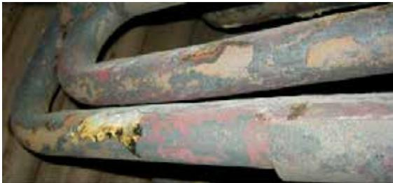
Fig. 9. SH2 after two years with ChlorOut..
