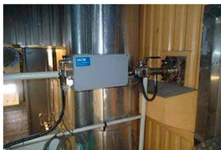
Fig. 4b. The spectrometer side of IACM in the boiler in Jordbro.
