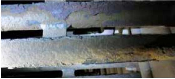
Fig. 7. Highly corroded tubes of SH2 after nearly four years without an additive.
