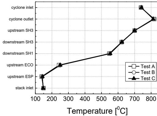
Fig. 8. Average flue gas temperature profiles during the tests A-C for some chosen locations along the convective pass.
