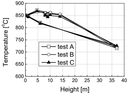
Fig. 5. Average bed temperature profiles in the CFB loop during tests A-C; boiler load: 100%.
