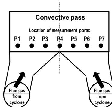
Fig. 3. The location of measurement ports across the horizontal flue gas duct.
