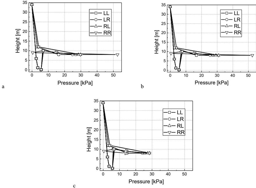
Fig. 4. Some chosen bed pressure profiles in the CFB loop during tests A-C; boiler load: 100%.
