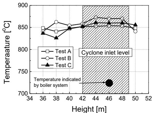
Fig. 6. Temperature profile along the combustion chamber in the upper section of the furnace for the tests A-C for a chosen measurement port. The black dots refer to the temperature values determined by boiler control system.
