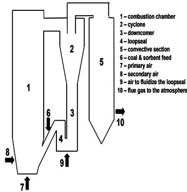
Fig. 1. Schematics of the commercial CFB boiler system.
