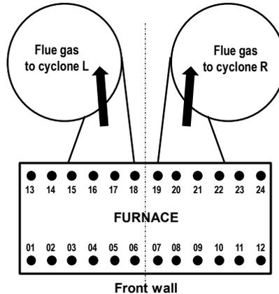
Fig. 2. Top view of the location of measurement ports across the boiler combustion chamber.
