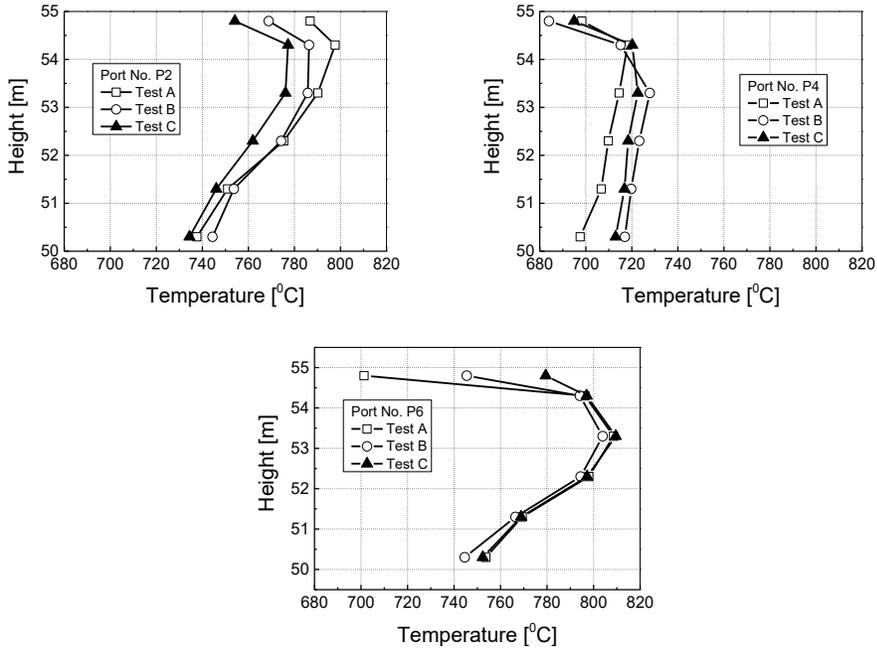
Fig. 7. Temperature profiles along the height of the inlet to the convective pass during the tests A-C for some chosen measurement ports. Boiler load: 100%.
