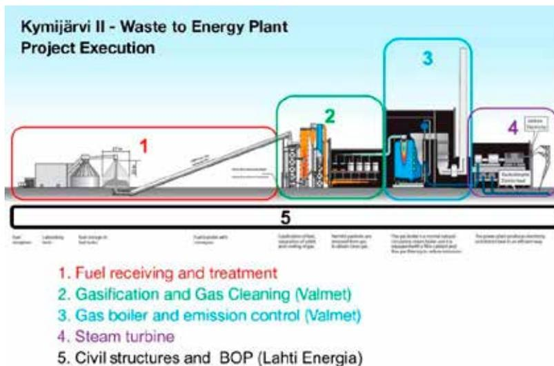
Fig. 6. Schematic structure of the Kymijärvi II plant
