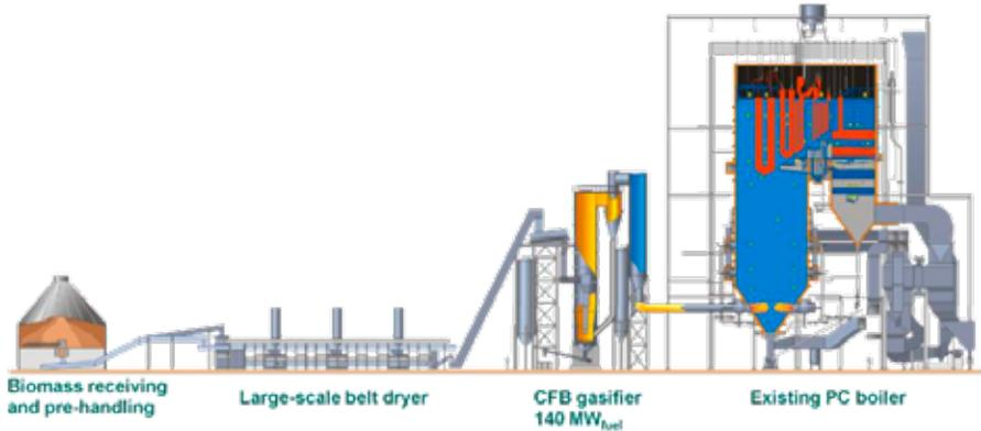
Fig. 5. The Vaskiluoto gasification plant
