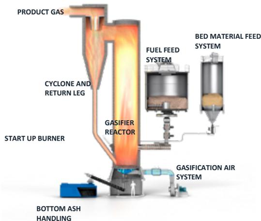
Fig. 3. Principal structure of the Valmet CFB gasifier
