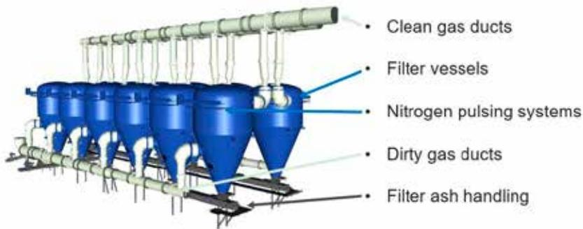
Fig. 7. Ceramic filter unit in the Kymijärvi II plant. Two parallel lines, each containing six modules. Each line serves one gasifier.
