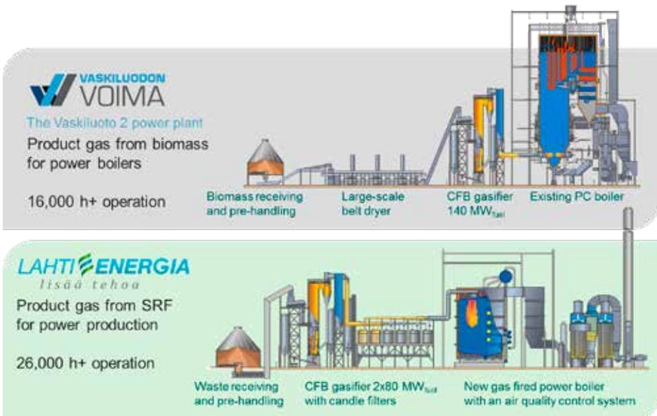
Fig. 1. Schematic of the presented CFB Gasification plants
