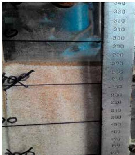
Fig. 6 – Picture of bed (90%  $Al_2O_3$  of 0.35 mm fraction, 10% sand).
