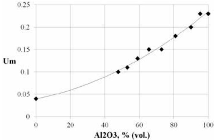
Fig. 2. Minimal fluidization velocity against the volume fraction of Al<sub>2</sub>O<sub>3</sub>.
