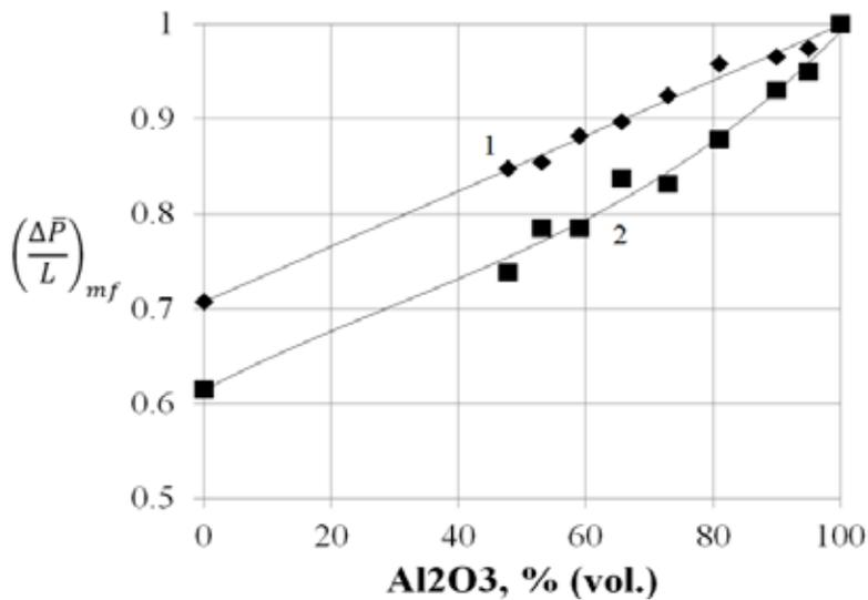
Fig. 3. Relative pressure gradient at minimal fluidization against the volume fraction of Al<sub>2</sub>O<sub>3</sub>.
