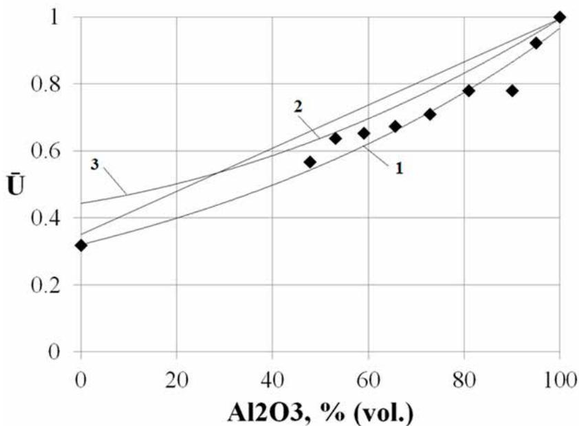
Fig. 4. The relative minimal fluidization velocity against the volume fraction of small fraction Al<sub>2</sub>O<sub>3</sub> in a mixture with sand. 1 - experimental data, 2 - according to eq. (7), 3 - according to eq. (1).
