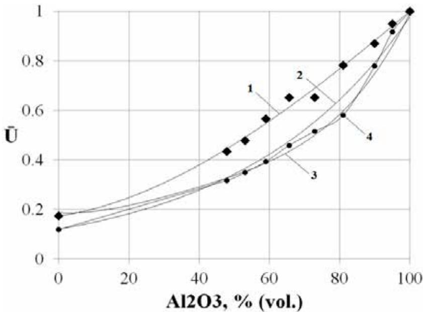
Fig. 5. The relative minimal fluidization velocity against the volume fraction of large fraction  $\text{Al}_2\text{O}_3$  in a mixture of sand for a large fraction of  $\text{Al}_2\text{O}_3$ . 1 - experimental data, 2 - according to eq. (7), 3 - according to eq. (1), 4 - according to eq. (7) with experimental value of real density of mixture.
