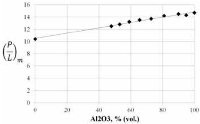
Fig. 1. The pressure gradient at the minimal fluidization against the volume fraction of Al<sub>2</sub>O<sub>3</sub>.
