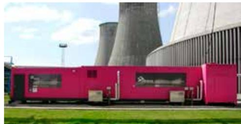
Figure 9e. Mobile VPSA-CO<sub>2</sub> unit.
