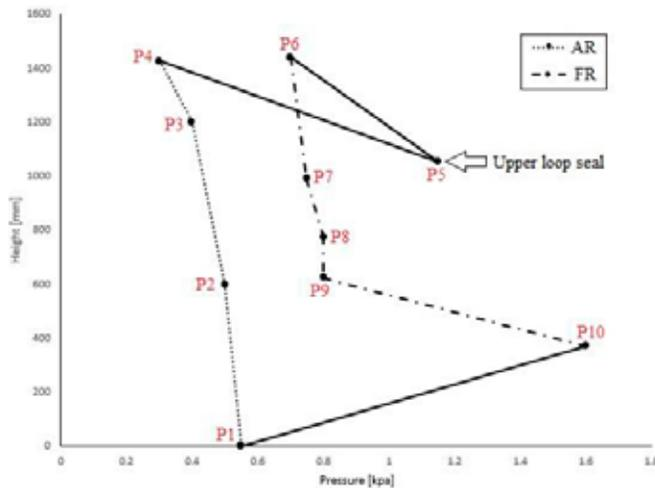
Fig.4. Pressure profile measured under standard operating condition
