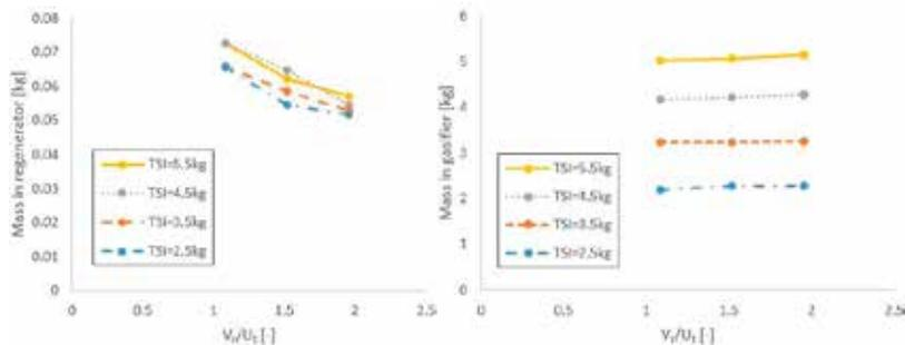
Fig.8. Mass distribution with different TSI and gas flow rate in regenerator
