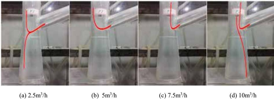
Fig.6. The route of discharging solids from upper loop-seal under different gas low rate in gasifier
