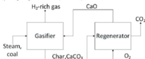
Fig.1. The schematic description of coal/CaO/steam system
