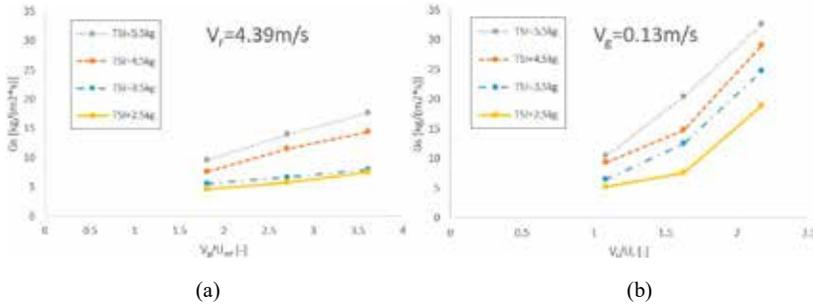
Fig.7. Solid circulation rate under different total solid inventories against increasing fluidization number
