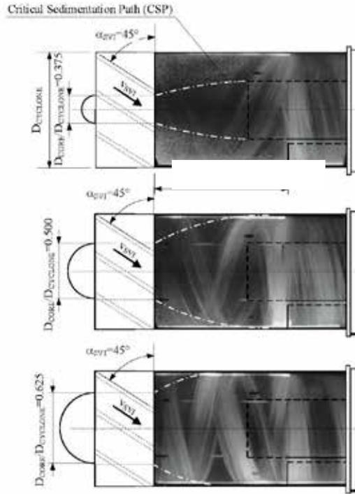
Fig. 5. Particle flow patterns inside the separation chamber of a uniflow cyclone with three different core diameter
