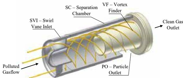
Fig. 1. Depiction of a uniflow cyclone and its flow field pattern.
