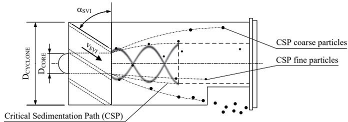
Fig. 4. Setup for dedusting tests and determination of the critical sedimentation path (CSP) inside the separation chamber (SC).
