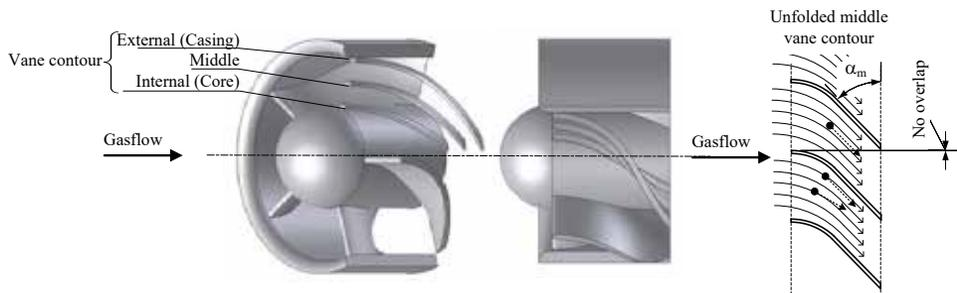
Fig. 3. Depiction an unfolded standard swirl vane inlet (SVI) of a uniflow cyclone.
