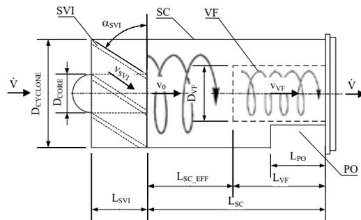
Fig. 2. Major geometric design parameters of a uniflow cyclone.
