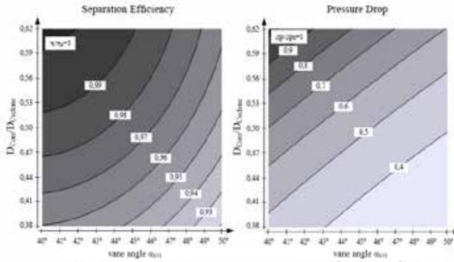
Fig. 7. Correlation of vane angle and separator performance, s. *Kraxner* (2013)
