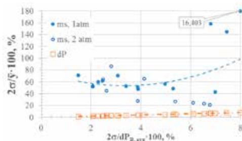
Figure 6. Relationship between scaled standard deviation in solids flow,  $\dot{m}_s$ , with that in the riser pressure differential,  $dP_r$ , for TR tests.
