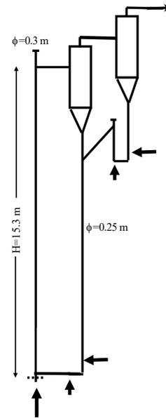
Figure 1. Schematic of NETL cold flow CFB
