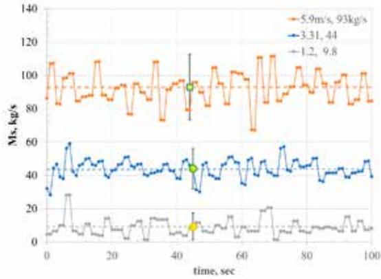
Figure 4. Time series solids flow rates for tests using glass beads TR26, TR32, and TR35 taken at 1.2 m/s in the fast fluidized, and 3.3, and 5.9 m/s in the core annular flow regimes, respectively.
