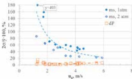
Figure 5. Comparison the scaled standard deviation in  $\bar{y}$  - i.e. both solids flow,  $\dot{m}_s$ , and riser pressure differential,  $dP_r$ , for TR tests.
