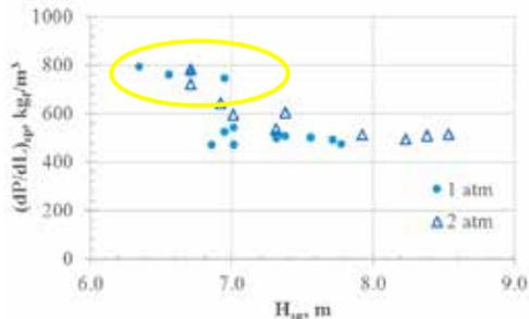
Figure 3. Apparent standpipe bed density for glass bead TR tests and its relationship with standpipe height.
