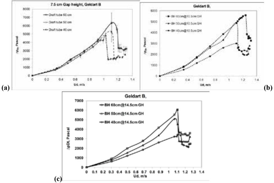
Fig 6. Pressure profiles for 40, 50 and 60 cm bed heights consisting Geldart B particles ICFB in the (a) draft tube (b) gap height of 10.5 cm and draft tube pressure (c) gap height of 14.5 cm and draft tube pressure
