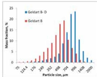
Fig. 1 Particle size distribution of silica particles.
