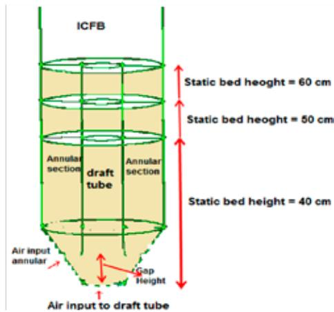
Fig. 4 ICFB experimental configuration schematic view
