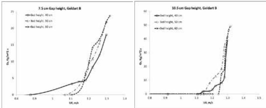
Fig 7. Solids circulation rate profiles for 40, 50 and 60 cm bed heights consisting Geldart B particles ICFB at different gap heights 7.5 cm and 10.5 cm
