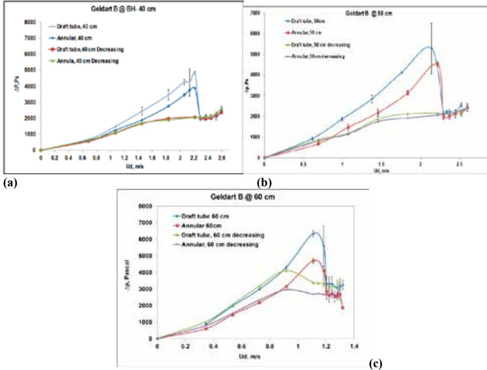
Figure 5 Pressure drop  $\nu_s$  superficial flow curve for (a) Bed height 40 cm (b) Bed height 50 cm and (c) Bed height 60 cm beds consisting of Geldart group B particles.
