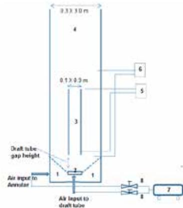
Fig 2. Schematic diagram of ICFB section. (1) annular air box (2) draft tube distributor (3) draft tube (4) ICFB (5) draft tube pressure measuring ports (6) annular bed pressure measuring ports (7) compressor (8) Air control valve
