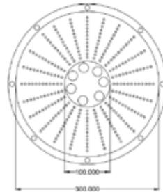
Fig. 3 Draft tube and annular distributor's dimensions in mm
