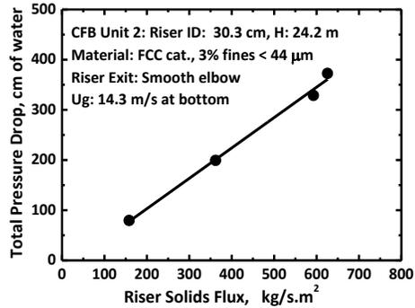
Fig. 15. Total riser  $\Delta P$  versus solids flux in CFB Unit 2 for  $U_g = 14.3$  m/s.
