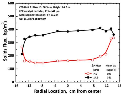
Fig. 9. Radial solids flux profiles at  $z = 13.2$  m in CFB unit 2 riser for two solids circulation fluxes at  $U_g = 15.2$  m/s.
