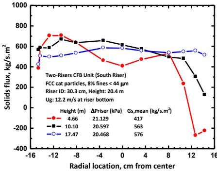
Fig. 13. Radial solids flux profiles at three axial locations in the south riser of the Two-Risers CFB unit at  $U_g = 12.2$  m/s and  $G_s$  of  $\sim 570$  kg/s-m<sup>2</sup>.
