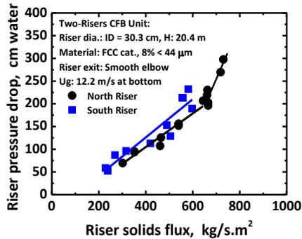
Fig. 16. Total riser  $\Delta P$  versus solids flux in the 2-Risers unit for  $U_g = 12.2$  m/s.
