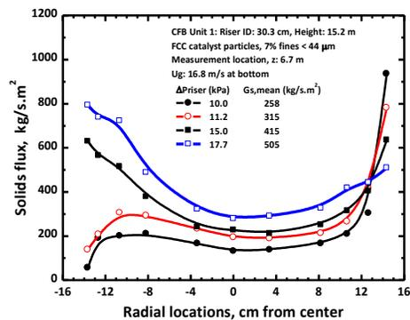
Fig. 7. Radial solids flux profiles at  $z = 6.7$  m in the CFB unit 1 riser for  $U_g = 16.8$  m/s and various solids fluxes.
