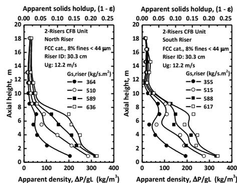
Fig. 5. Apparent density profiles in the North and South risers of the Two-Riser CFB unit at Ug = 12.2 m/s for various solids fluxes.
