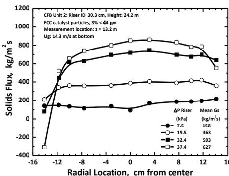
Fig. 8. Radial solids flux profiles at  $z = 13.2$  m in CFB unit 2 riser for  $U_g = 14.3$  m/s and various  $G_s$  values.
