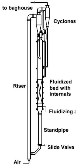
Fig. 1. Schematic drawing of CFB Unit 1. Riser ID = 30.3 cm and H = 15.24 m.
