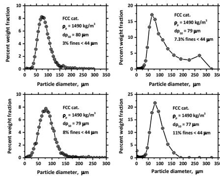
Fig. 4. Particle size distribution of FCC catalyst particles
