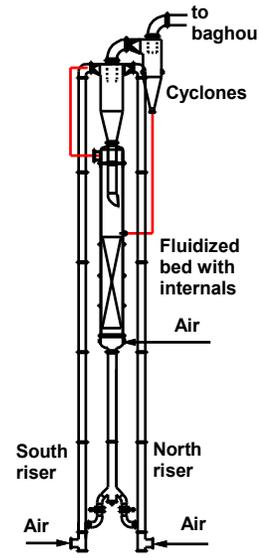
Fig. 3. Schematic drawing of the Two-Riser CFB Unit. Riser ID = 30.3 cm and H = 20.4 m.
