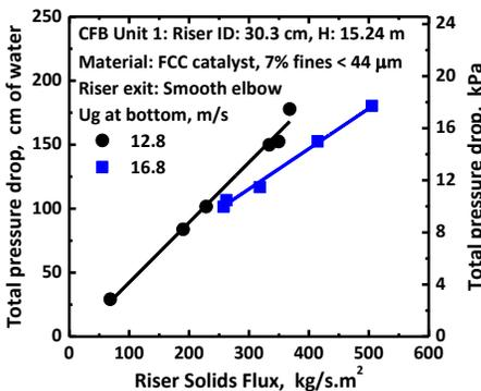
Fig. 14. Total riser  $\Delta P$  versus  $G_s$  in CFB Unit 1 for  $U_g = 12.8$  and  $16.8$  m/s.
