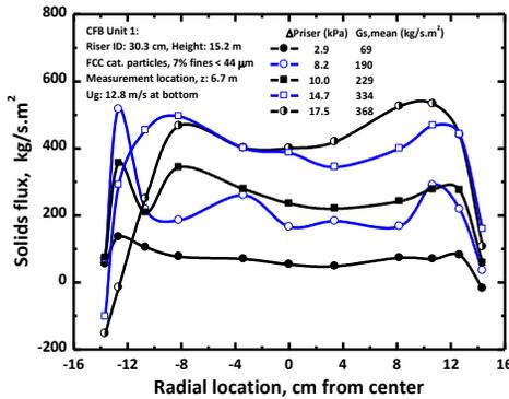
Fig. 6. Radial solids flux profiles at  $z = 6.7$  m in the CFB unit 1 riser for  $U_g = 12.8$  m/s and various solids fluxes.
