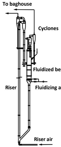
Fig. 2. Schematic drawing of CFB Unit 2. Riser ID = 30.3 cm and H = 24.2 m.
