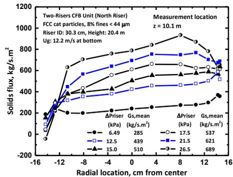
Fig. 11. Solids flux profiles at  $z = 10.1$  m in the North riser of the Two-Risers CFB unit for  $U_g = 12.2$  m/s and various solids fluxes.
