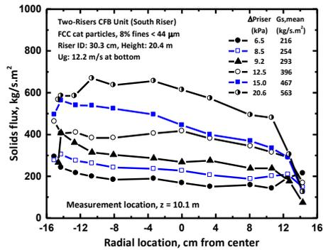
Fig. 10. Solids flux profiles at  $z = 10.1$  m in the South riser of the Two-Risers CFB unit for  $U_g = 12.2$  m/s and various solids fluxes.
