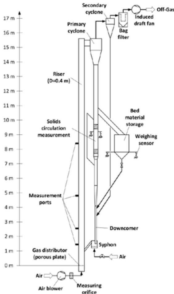
Fig. 1. Flow sheet of the circulating fluidized bed setup.
