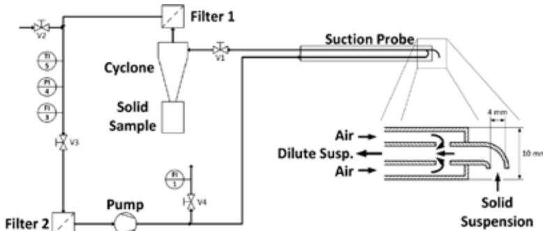
Fig. 4. Flow sheet of the suction probe system for solid sampling.
