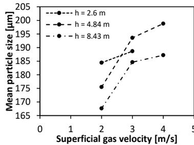
Fig. 7. Influence of superficial velocity and height from distributor on mean particle size.
