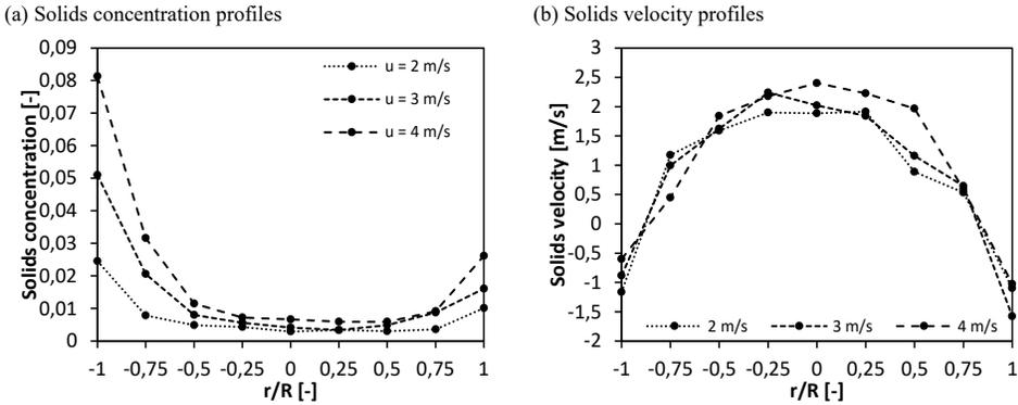
Fig. 5. Radial solids (a) concentration and (b) velocity profiles at a height of 1.5 m from air distributor.
