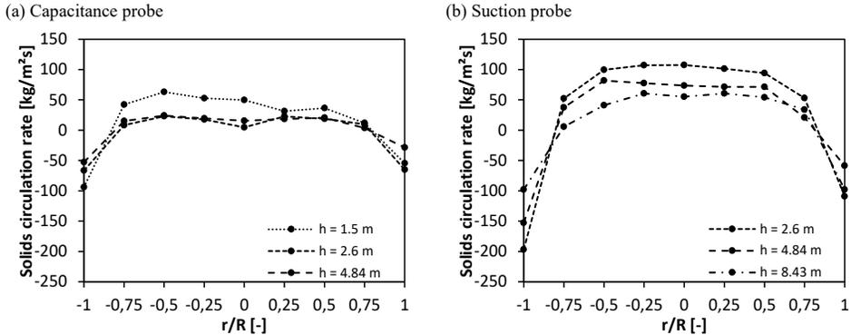
Fig. 6. Radial solids circulation rate profiles at a superficial velocity of 3 m/s at different heights measured (a) by capacitance probe and (b) by suction probe.
