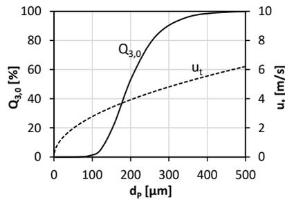
Fig. 2. Mass density distribution and terminal velocity of a single particle as functions of the particle size
