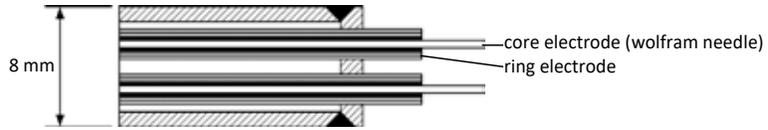
Fig. 3. Setup of the capacitance probe.
