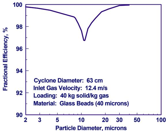
Fig. 30. Cyclone Efficiency vs. Particle Size With Indication of Small-Particle Clumping
