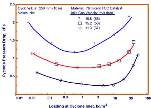
Fig. 1. The effect of loading on cyclone pressure drop
