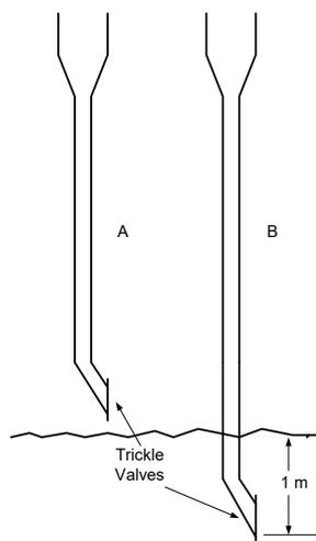
Fig. 26. Immersed and Non-immersed Trickle Valves
