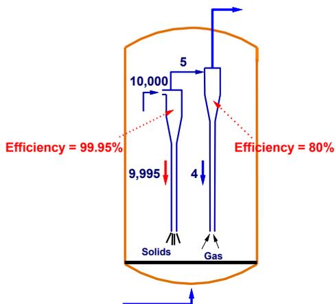
Fig 16. Relative loading in primary and secondary cyclones
