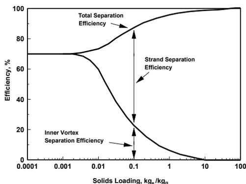
Fig. 9. Muschelknautz *et al.*, 1996 critical loading plot
