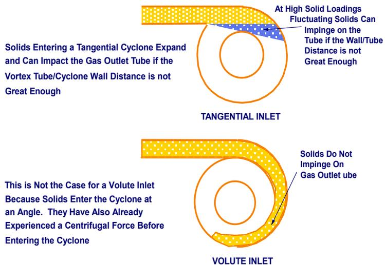
Fig. 7. Tangential and Volute Inlet Operation at High Solids Loading
