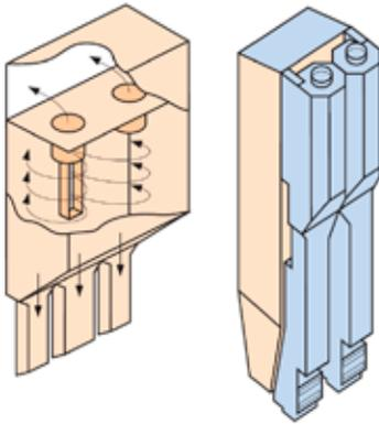
Fig. 13. Compact Solids Separators
