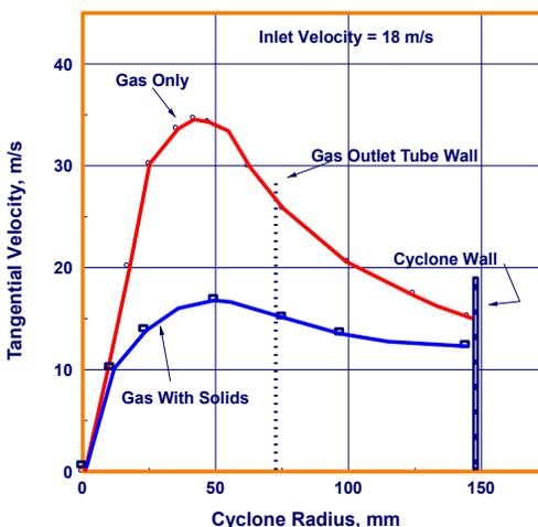
Fig. 2. Cyclone tangential velocity with and without solids flow in the cyclone
