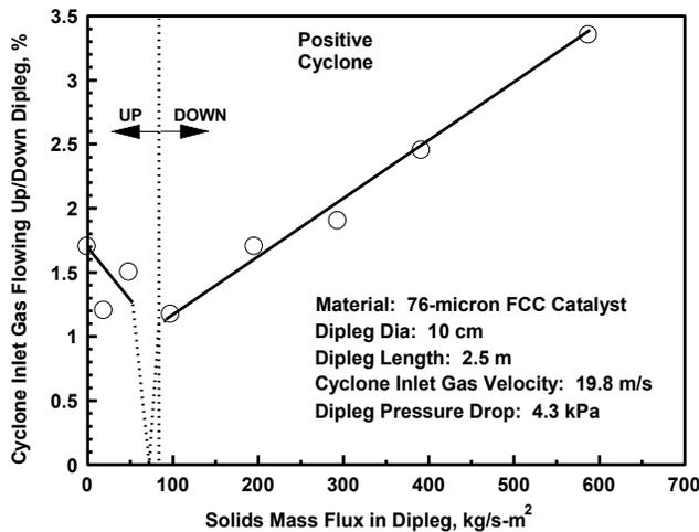
Fig. 24. The Effect of Solids Mass Flux in the Dipleg on the Direction of Gas Flow for FCC Catalyst
