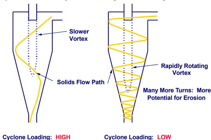
Fig. 17. Solids flow in low- and high-loaded cyclones
