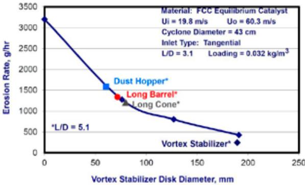
Fig 19. Effect of Flat Plate Vortex Stabilizer Diameter on Erosion Rate
