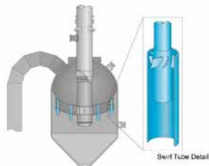
Fig. 4. Third-Stage Separator (Shell type) with axial inlet swirl tubes
