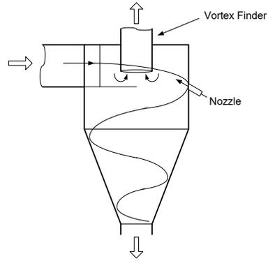
Fig. 12. Gas nozzle to regulate solids flow out of a cyclone
