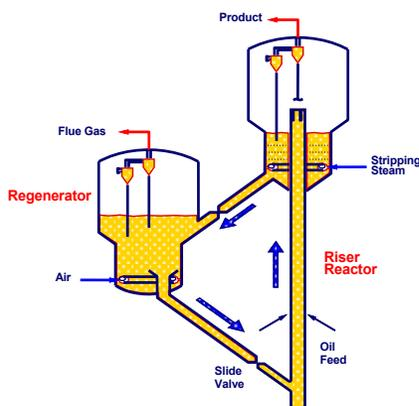
Fig. 3. Schematic Drawing of a Side-by-Side FCC Unit
