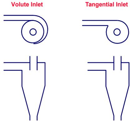
Fig. 6. Schematic Drawing of Tangential and Volute Cyclone Inlets
