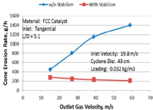
Fig.20. Cone Erosion Rate vs. gas velocity in the GOT for a flat-plate vortex stabilizer
