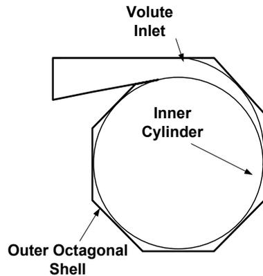
Fig. 14. Schematic Drawing of an Octagonal Cyclone
