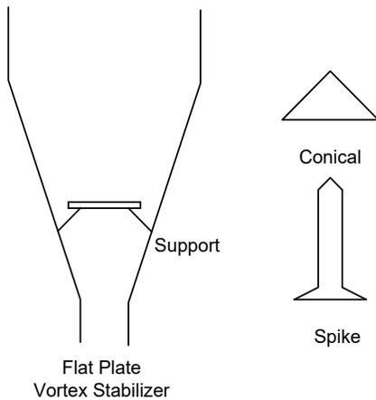
Fig. 21 Types of Vortex Stabilizers
