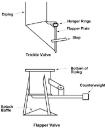
Fig. 23. Schematic Drawing of Trickle and Counterweighted Flapper Valves
