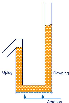
Fig. 28. Schematic Drawing of a Loop Seal
