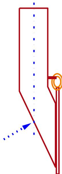
Fig. 27. Optimum Aeration Location for a Trickle Valve
