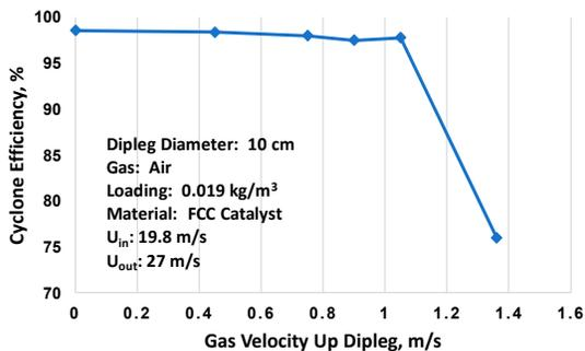
Fig. 25. Cyclone Efficiency vs. Gas flow Up the Dipleg
