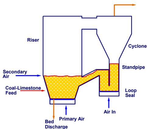
Fig 5. Schematic Drawing of a CFBC
