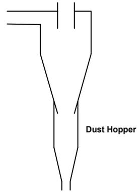
Fig. 18. Cyclone with Dust Hopper
