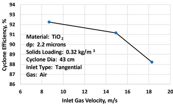
Fig. 29. Cyclone Efficiency vs. Inlet Gas Velocity for TiO<sub>2</sub>
