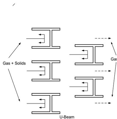
Fig. 22. Top View of U-beams
