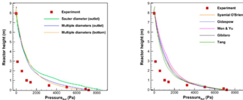
Figure 4: Pressure profiles left hand side: Influence of experimental PSD using Syamlal O'Brien drag model, right hand side: Influence of drag models using PSD at outlet
