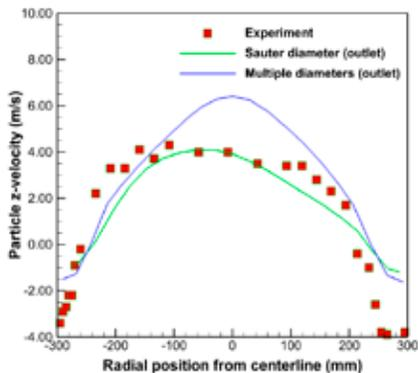
Figure 6: Time averaged parcel velocities using Syamlal O'Brien drag model in comparison with the experiment
