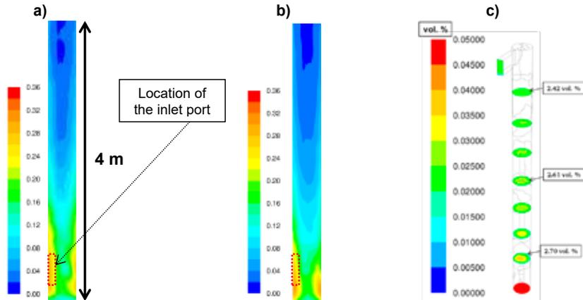
Figure 5: Comparison of time averaged particle volume fraction using (a) Syamlal O'Brien (b) Tang et al. drag model; (c) Time averaged CO<sub>2</sub> concentration inside the reactor using Syamlal O'Brien drag model
