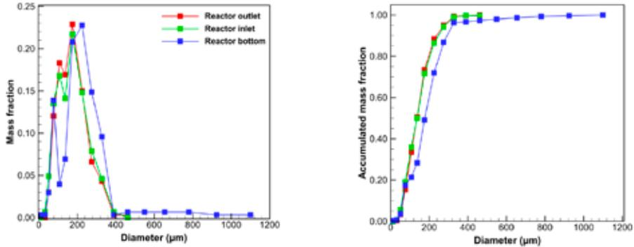
Figure 1: Particle size distribution at different extraction positions in the experiment
