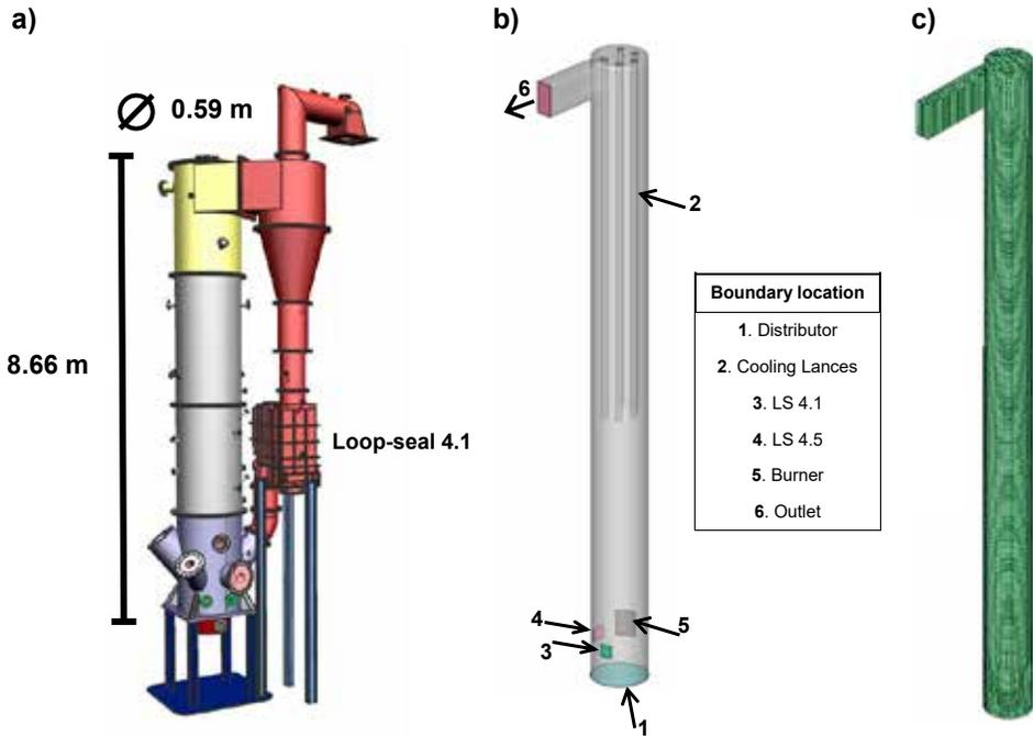
Figure 2: Carbonator reactor simplification a) CAD drawing of real sized model b) CFD geometry of riser only c) Discretization of the geometry
