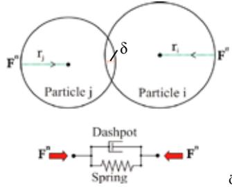
Figure 3: Spring-Dashpot collision law
