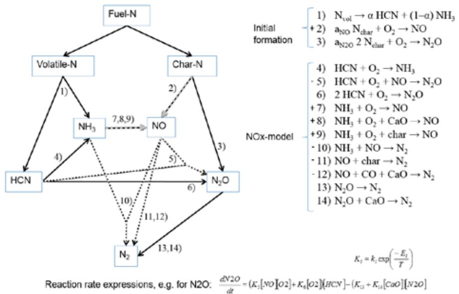
Fig.3. NOx model reactions in CFB3D model.
