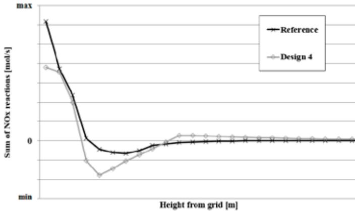
Fig.6. Total NOx reaction rates [mol/s] as function of furnace height (only part of the furnace).
