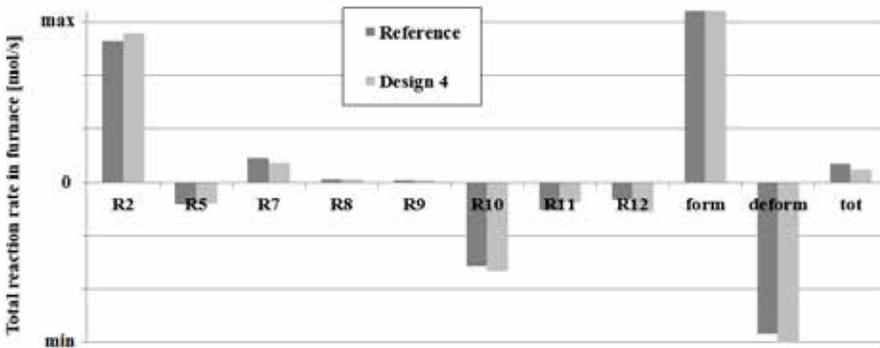
Fig.5. Total reaction rates [mol/s] in furnace of individual NO<sub>x</sub> reactions.
