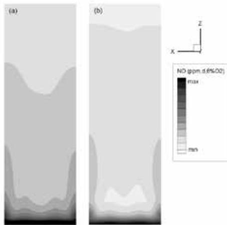
Fig.8. Modeled NO<sub>x</sub> concentration [ppm,d,6%O<sub>2</sub>] for (a) Reference (b) Design 4.
