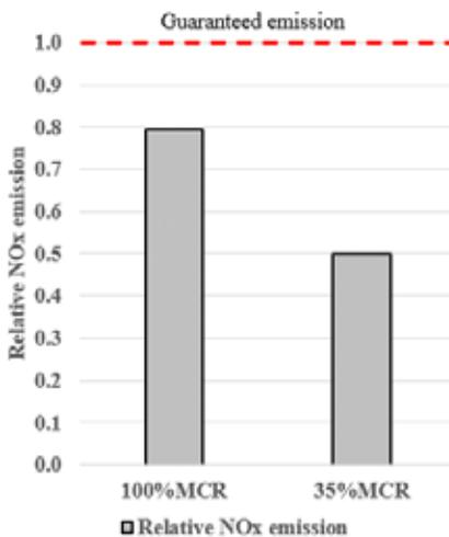
Fig.10. Realized NO<sub>x</sub> emission compared to the guarantee.
