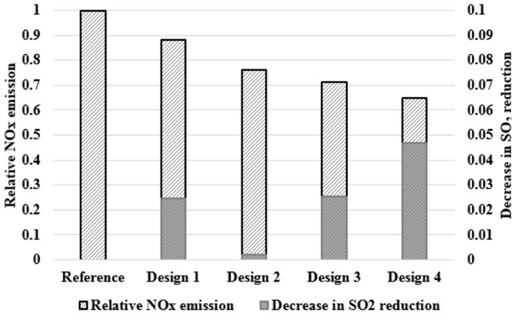
Fig.4. NO<sub>x</sub> reductions on a coal fired CFB unit with different design changes.
