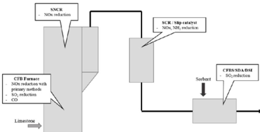
Fig.1. Flow diagram of total optimization of emissions in CFB boiler.
