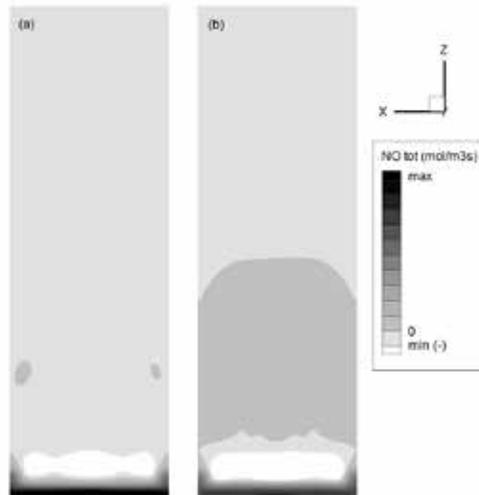
Fig.7. Modeled total NOx reaction rate for (a) Reference (b) Design 4.
