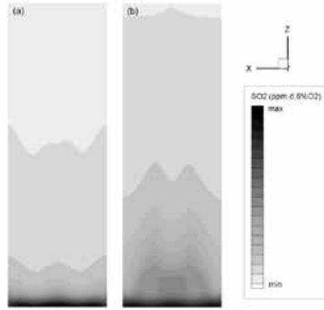
Fig.9. Modeled SO<sub>2</sub> concentration [ppm,d,6%O<sub>2</sub>] for (a) Reference (b) Design 4.
