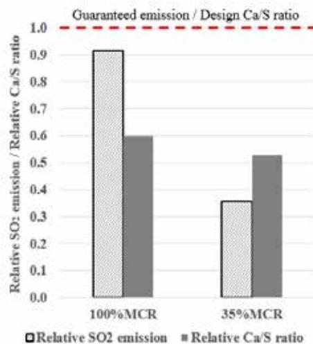
Fig.11. Realized SO<sub>2</sub> emission and Ca/S ratio compared to guarantee / design value.
