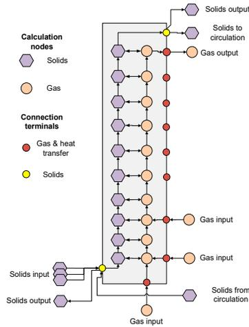
Fig. 2. Schematic picture of the furnace nodalisation and connections.
