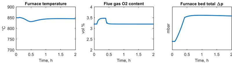
Fig. 7. Transient simulation from 100 % to 80 % load. Furnace average temperature, flue gas  $O_2$  content, and total pressure drop over the furnace bed.
