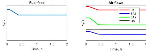
Fig. 6. Transient simulation from 100 % to 80 % load. Fuel feeding and air flows.
