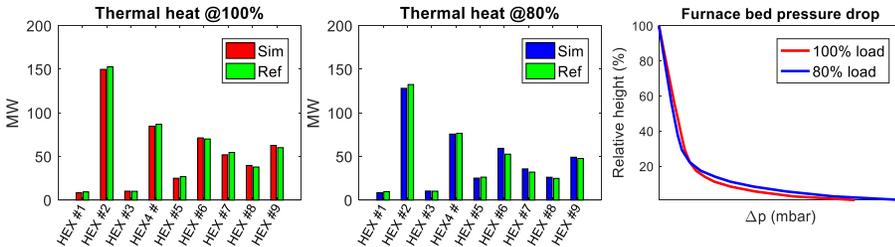
Fig. 5. Comparison of the simulated heat exchanger duties with the design references in steady state at 100 % (left) and 80 % (middle) load; Simulated furnace bed pressure difference profile at 100 % and 80 % load (right).
