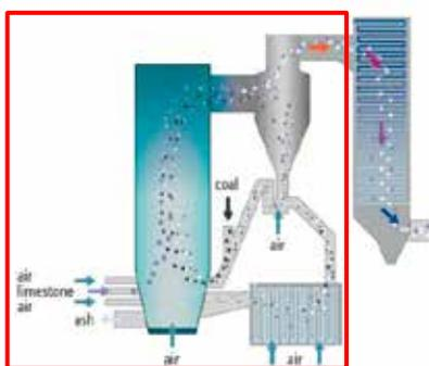
Fig. 1. Schematic picture of the boiler type (only the framed part was addressed in this study).
