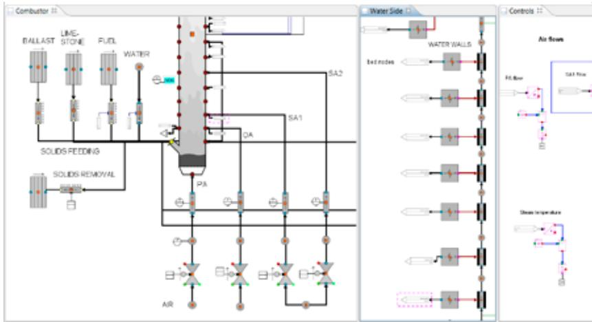
Fig. 4. Views to the model diagrams: solids and air feeding to the furnace (left), part of the water walls (middle), and control loops (right). The highlighted reference flags (see right side of the furnace, and the lowest water wall tube section) show an example, how the model continues from a diagram to another.
