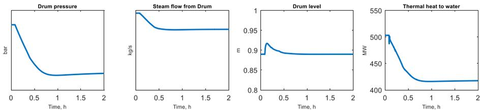
Fig. 8. Transient simulation from 100 % to 80 % load. Drum pressure and level, steam flow and thermal heat to water.
