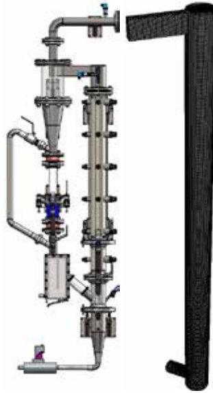
Fig. 1. The laboratory-scale CFB device (left) and the computational mesh (right).
