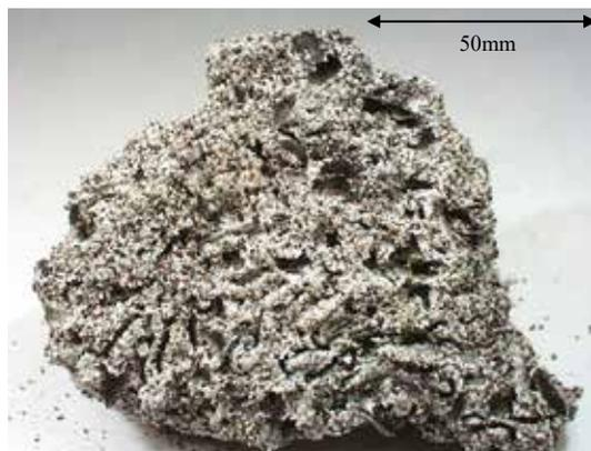
Fig. 1. Photograph of a large sand agglomerate after pilot-scale FBC of biomass (Chirone et al., 2006).
