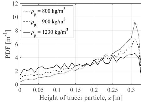
Fig. 9: Modelling results of vertical position of the tracer, comparing different particle densities for  $H_o = 0.3$  m,  $u_o - u_{mf} = 0.37$  m/s,  $D_p = 0.05$  m.
