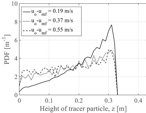
Fig. 6: Modelled results of the axial distribution of the fuel tracer at different fluidisation velocities.  $H_o = 0.3 \text{ m}$ ,
