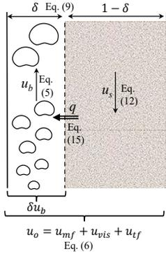
Fig. 1: Schematic of two phase model.
