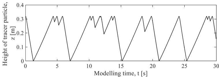
Fig. 4: Axial location of the tracer over 30 seconds of modelling time.
