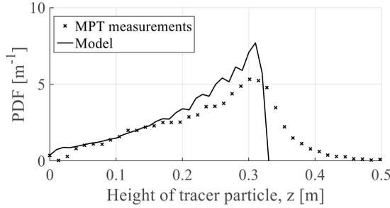
Fig. 5: Comparison of modelling results with MPT data (Köhler et al., 2017) using vertical position of the tracer.
