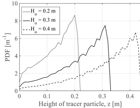
Fig. 7: Modelled results of the axial distribution of the fuel tracer at different fixed bed heights.
