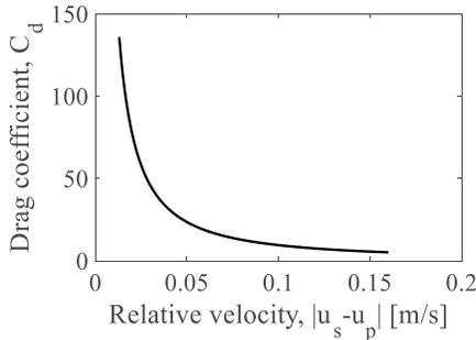
Fig. 3: Drag coefficient,  $C_d$ , as function of relative particle velocity,  $u_p - u_s$ .
