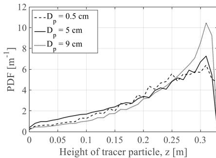
Fig. 8: Modelling results of vertical position of the tracer, comparing different particle diameters for  $H_o = 0.3$  m,  $u_o - u_{mf} = 0.19$  m/s,  $\rho_p = 1230$  kg/m<sup>3</sup>.
