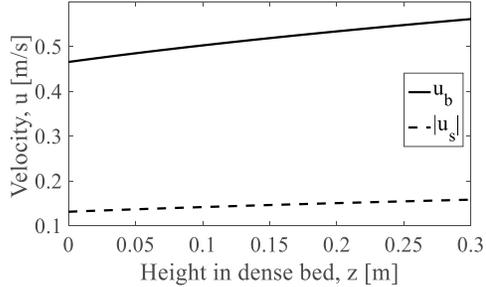
Fig. 2: Bubble velocity,  $u_b$ , and emulsion velocity,  $u_s$ , over bed height  $z$ .
