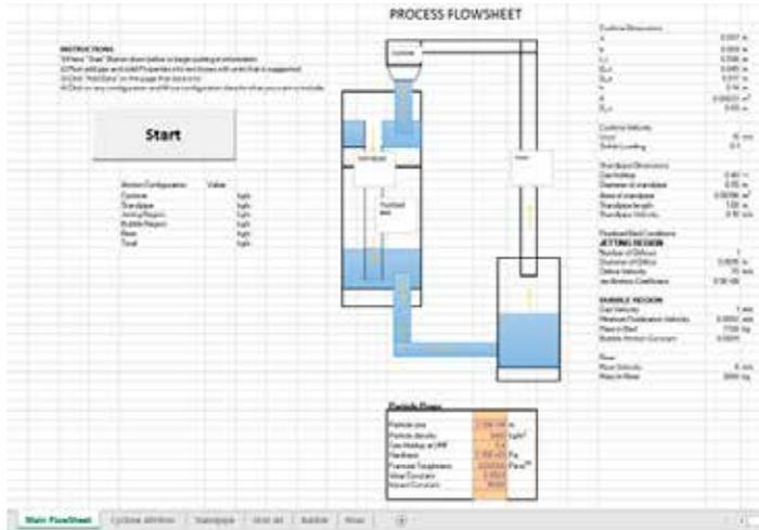
Fig. 2- Screenshot of the spreadsheet main flowsheet. Contains all input information, instructions for running the model, and results. Additional sheets containing individual calculations for each configuration are also shown.
