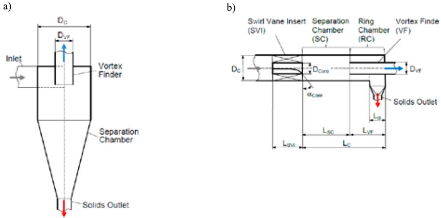
Fig. 1. Main design parameter of a standard reverse-flow cyclone (a) and a uniflow cyclone with swirl vane inserts (b).  $D_C$ : cyclone diameter,  $L_C$ : cyclone length,  $D_{VF}$ : vortex finder diameter,  $L_{VF}$ : vortex finder length,  $D_{Core}$ : core diameter,  $L_B$ : bunker length,  $\alpha_{core}$ : guide vane angle at the core.
