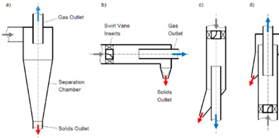
Fig. 2. Schematic illustration of a standard cyclone (a) and uniflow cyclones with axial inlet and horizontal (b), vertical downward (c) and vertical upward orientation (d).
