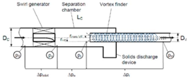
Fig. 4. Calculation of the pressure drop of uniflow cyclones.
