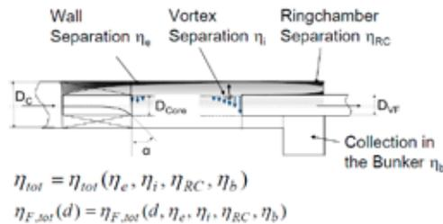
Fig. 3. Overall structure of the separation process in a uniflow cyclone.
