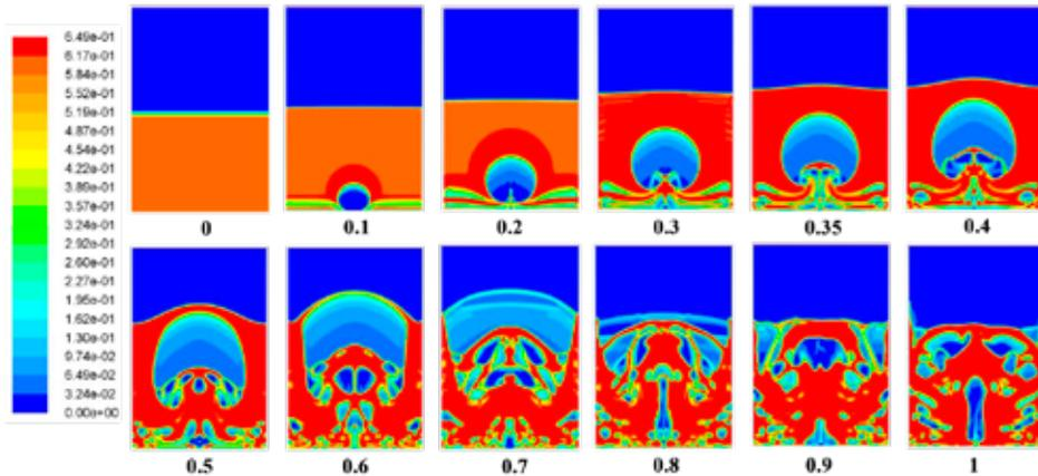
Fig.2: Evolution of bubble with time (seconds) by central gas jet in bubbling fluidized bed predicted by Beetstra drag model.
