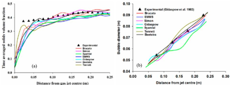
Fig. 3: CFD predicted (a) time averaged solids volume fraction (b) bubble diameter along the axial direction from jet centre in bubbling fluidized bed.
