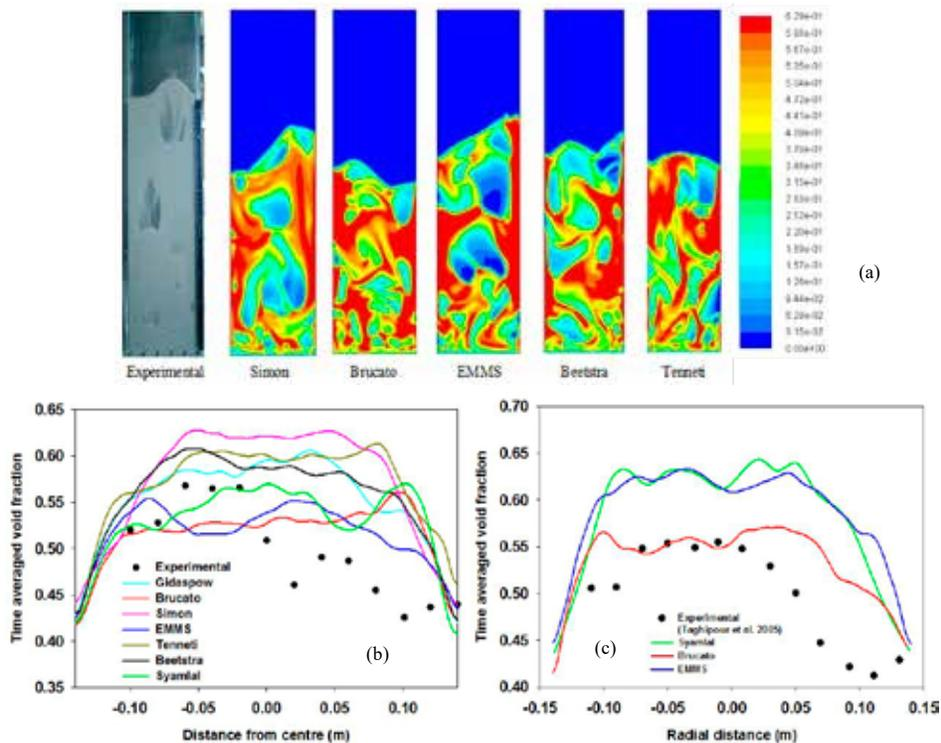
Fig.5: Comparison of CFD predicted (a) mean solids volume fraction contours and (b) time averaged mean void fractions along the radial direction at an axial height of 0.2 m, velocity of 0.38 m/s in a uniformly fed freely bubbling fluidized bed for different drag models.
