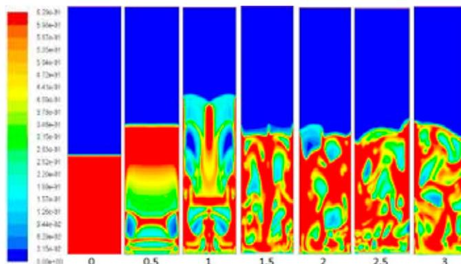
Fig.4: variation of CFD predicted solids volume fraction profiles at different time in turbulent fluidized bed ( $U = 0.38$  m/s, drag function: Brucato).
