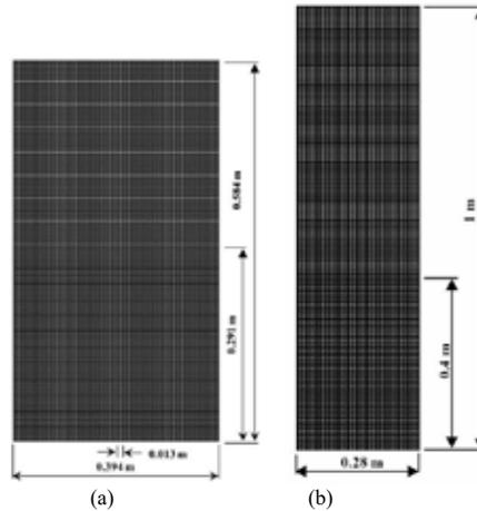
Fig. 1 Meshes used for (a) bubbling fluidized bed with central gas jet and (b) uniformly fed turbulent fluidized bed.
