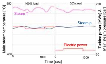
Fig. 3. Primary grid support in a 300 MWth CFB firing lignite at full and minimum load (based on Kovacs et al., 2015)
