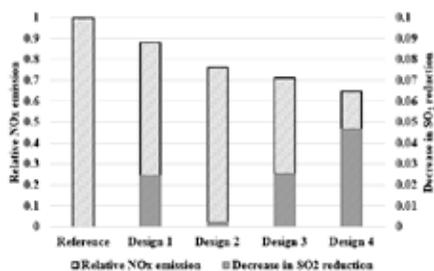
Fig.2. NOx reductions in a coal fired CFB unit using different design changes (Kipinoinen et al., 2017)
