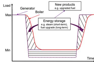
Fig. 4. Example of increased plant flexibility by storing/utilizing excess energy from the ramp-down phase to boost the ramp-up phase.
