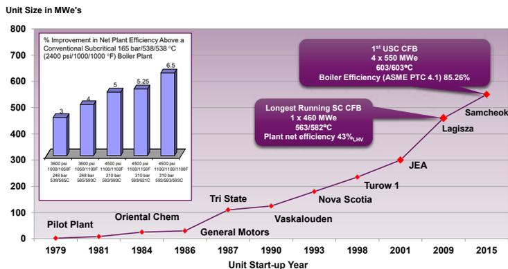
Fig. 1. Increase of plant efficiency with CFB boilers from the 1980s, and advantage of SC steam data.
