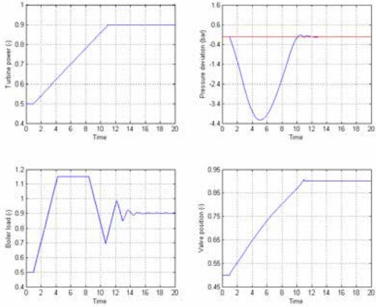
Figure 6 BPCP with optimized main steam pressure behavior.
