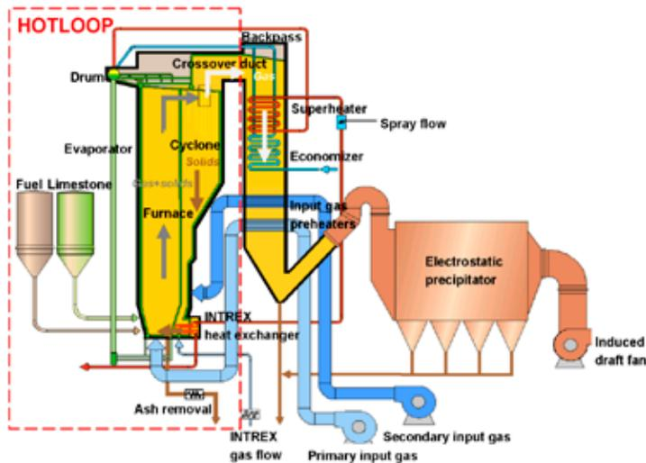
Figure 1 Operation schematic of a CFB boiler.
