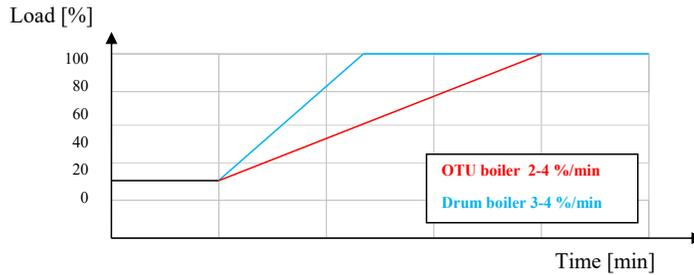
Figure 2 Typical load change capability of different CFB boilers and turbine.
