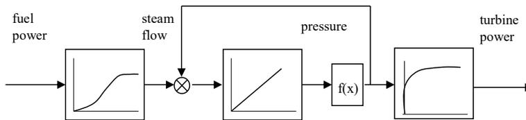
Figure 3 Simplified representation of the dynamic relationships in boiler/turbine process.
