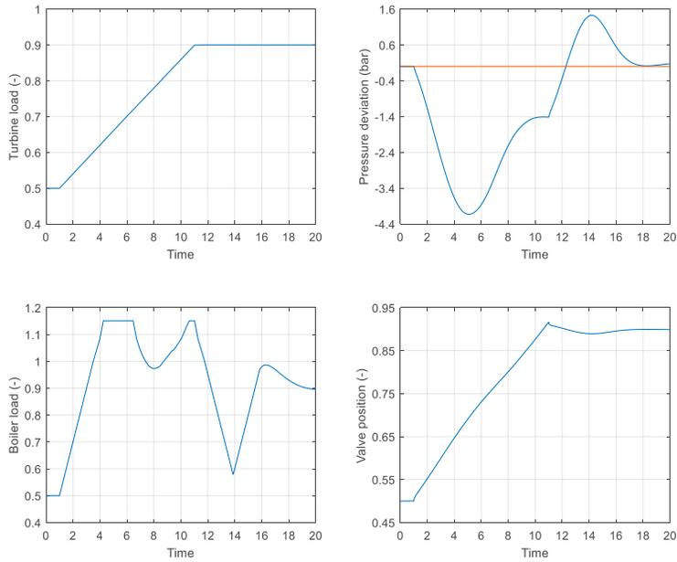
Figure 7 Approximation of the BPCP with two PID feedback controllers.
