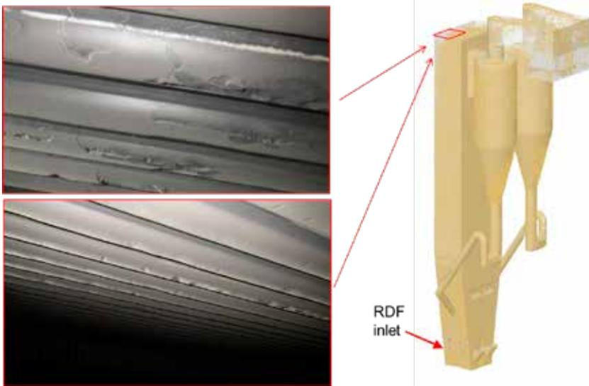
Fig. 6. Wuppertal Elberfeld plant: Specific Tube Damages at the Roof
