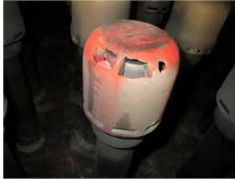
Fig. 2. Damaged Primary Air Nozzle due to External Wear
