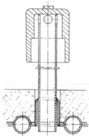
Fig. 1. Cross section of a typical primary air nozzle
