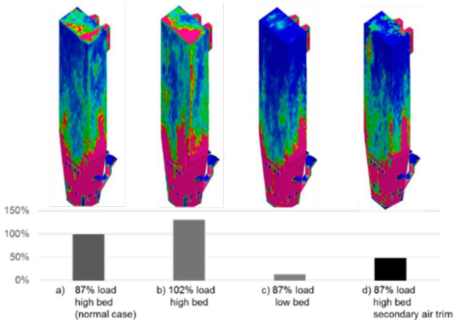
Fig. 8. Wear scenario simulations: plot of wall/roof wear intensity and normalized values for roof wear
