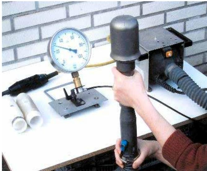
Fig. 3. Device for the Measurement of internal Pressure Drop of individual Primary Air Nozzles
