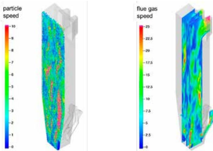
Fig. 7. Instantaneous values of particle speed (left, max value 10 m/s) and flue gas speed (right, max value 25 m/s)
