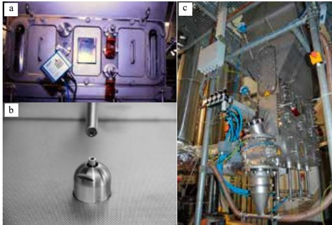
Fig. 3. Photos of the samplers and the installed inline probe (a), the nozzle within the process chamber (b) and the used pilot plant granulator (c)
