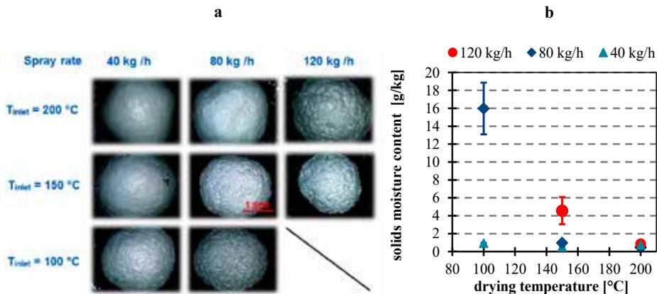
Fig. 4. Images of the particle surfaces of the different products (a) and solids moisture content of the bulk material during the granulation process (b).
