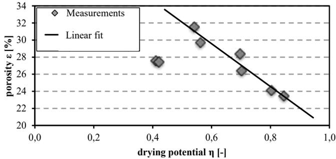
Fig. 7. Measured granule porosities in dependence of the drying potential of each granulation experiment. Neglecting the two experiments with drying potentials  $\eta$  less than 0.5 an additional linear fit was added.
