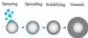
Fig. 1: Principle of the spray granulation process
