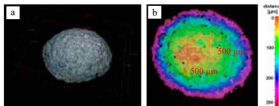
Fig. 5. Example for a created 3D-structure of a focus-variation measurement (a) and the height profile of the corresponding particle surface (b).
