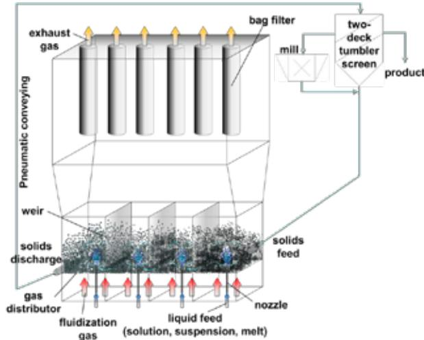
Fig. 2. Scheme of a multi-staged horizontal fluidized bed apparatus
