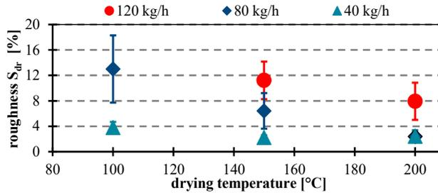
Fig. 6. Characterization of the surface roughness based on the ratio of the true volume to the projected volume  $S_{dr}$  of the granules, produced under different process conditions.
