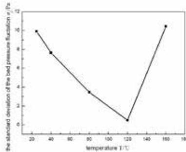
Fig.5. The standard deviation of the bed pressure fluctuation under different temperature at  $U-U_{mf}=2\text{cm/s}$
