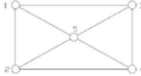
Fig.2. The distribution of pressure measurement points on a cross-section of fluidized bed
