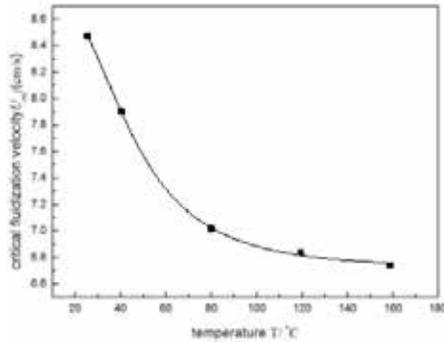
Fig.4. Regression curve between critical fluidization velocity and temperature
