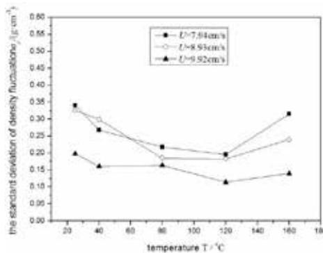
Fig.6. The fluctuation variance of the layer density of 40~60mm
