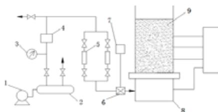
1-Roots blower 2-Air tank 3-Manometer 4-Filter 5-Flow meter 6-Air duct heater
