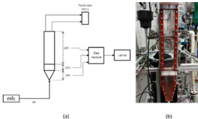
Figure 2:(a) Process and instrumentation diagram (b) cold flow spouted bed unit.
