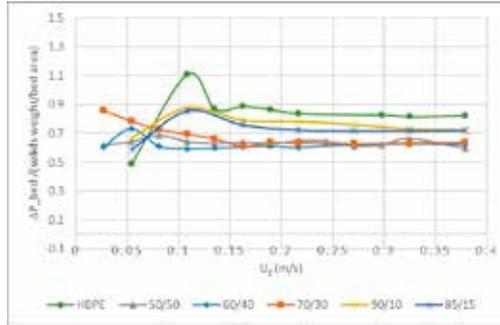
Figure 6: Normalized average pressure profiles for 4-inch beds of pure HDPE and HDPE/Hematite mixtures of 90/10, 85/15, 70/30, 60/40 and 50/50.
