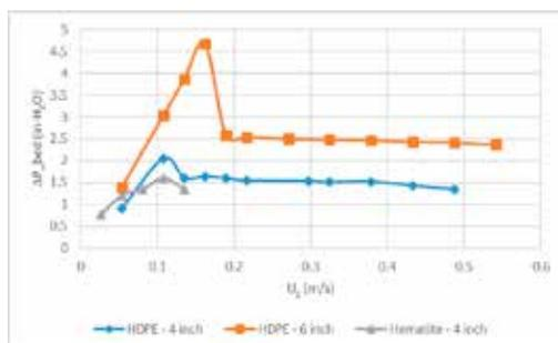
Figure 3: Average Pressure Profiles for various bed heights of unmixed HDPE and Hematite
