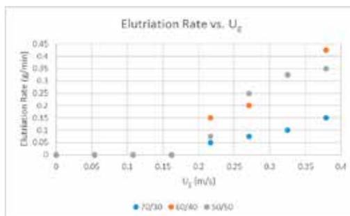
Figure 9: elutriation rate of hematite vs. superficial gas velocity,  $U_g$ , for the 70/30, 60/40, and 50/50 HDPE/hematite mixtures.
