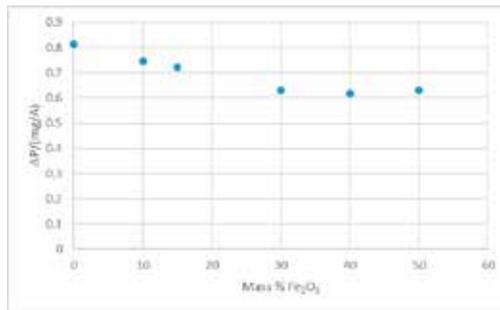
Figure 7: Average of normalized pressure values for all gas velocities beyond  $U_g > U_{mf, HDPE}$  versus mass percentage of cohesive  $Fe_2O_3$  powder in bed.
