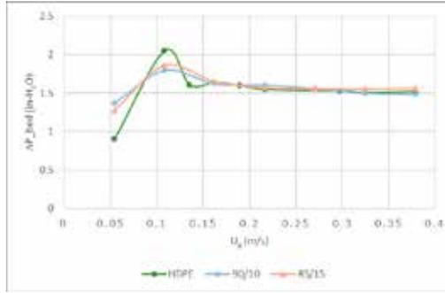
Figure 4: Average pressure profiles for 4-inch beds of pure HDPE and HDPE/Hematite mixtures of 90/10 and 85/15.
