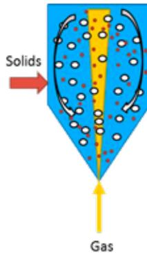
Figure 1: Conceptual diagram of a spouted bed
