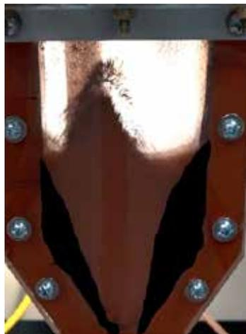
Figure 8: Image showing regions of apparent non-interactive particles (darker shaded areas) for the 50/50 HDPE/hematite mixture case. ( $u_g = 3.25$  m/s)
