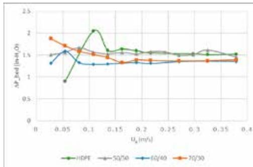
Figure 5: Average pressure profiles for 4-inch beds of pure HDPE and HDPE/Hematite mixtures of 70/30, 60/40 and 50/50.
