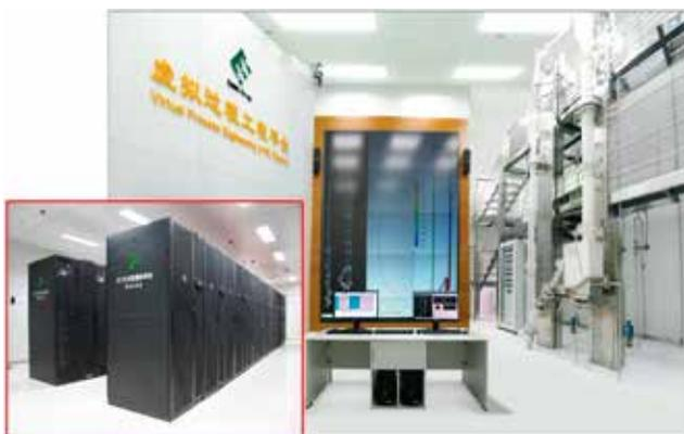
Fig. 6. Version 1.0 of VPE: On the right is an experimental unit. A screen of the same height as that of the unit is shown in the middle. A computer controls both the experiment and simulation to allow online comparison (Li et al., 2016)
