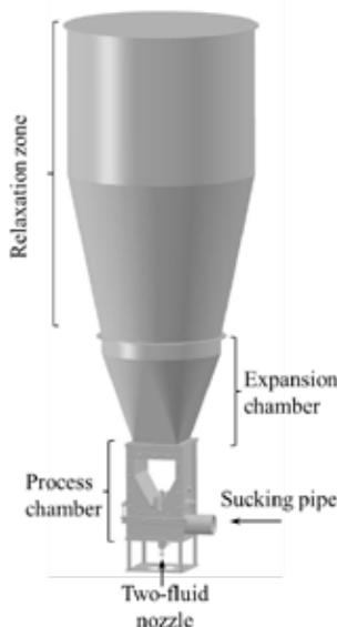
Fig. 2. Spouted bed for coating of fine particles.
