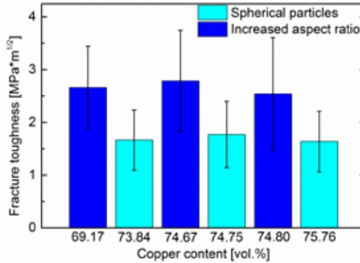
Fig. 5. Fracture toughness of different copper-polymer composites.
