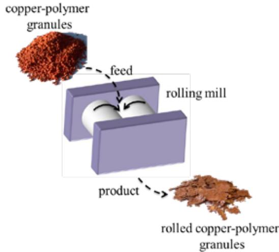
Fig. 3. Rolling step of coated copper particles.
