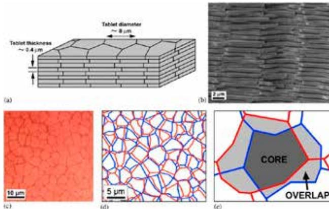
Fig. 1. Structure of nacre. (a) Schematic of the tablets arrangement in nacre; (b) scanning electron micrograph of a fracture surface in nacre; (c) top view of tablet tiling in nacre; (d) reconstitution of the arrangement of the tablets from one layer to the next; (e) core and overlap areas in the tablet arrangements (Barthelat et al., 2007).
