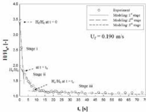
Fig. 5. Bed collapse curve for the MWCNT agglomerates;  $U_f = 0.190$  m/s.
