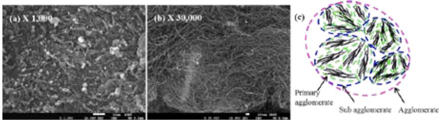
Fig. 1. SEM image of MWCNT agglomerates (a,b) and scheme of multi-agglomerate structure for MWCNT agglomerates (c).
