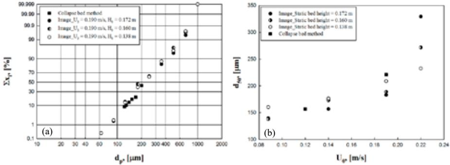
Fig. 6. (a) cumulative size distribution of MWCNT agglomerates obtained by collapse bed method and image analysis, (b) median diameter ( $d_{50}$ ) of MWCNT agglomerates determined by the image analysis and collapse bed methods.
