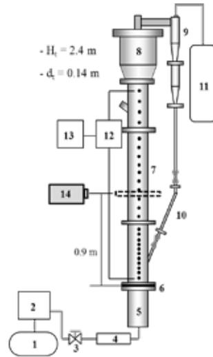
Fig. 2. Schematic diagram of experimental setup; 1 air compressor, 2 air dryer, 3. Pressure regulator, 4 mass flow controller, 5 windbox, 6 distributor, 7 fluidized bed, 8 expansion column, 9 cyclone, 10 standpipe, 11 bag filter, 12 pressure transducer, 13 recorder, 14 high speed camera.
