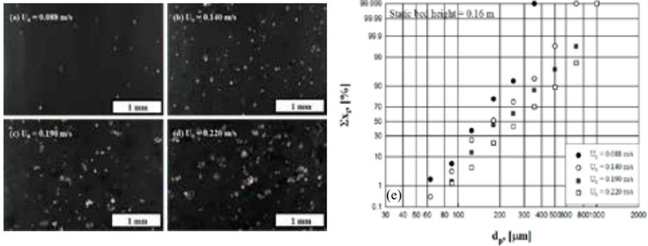
Fig. 4. (a-d) Photograph of MWCNT agglomerates (bright spots) in freeboard measured using high-speed camera; (a)  $U_0 = 0.088$  m/s, (b)  $U_0 = 0.140$  m/s, (c)  $U_0 = 0.190$  m/s, (d)  $U_0 = 0.220$  m/s; (e) Cumulative size distribution of MWCNT agglomerates in the freeboard measured using a camera.
