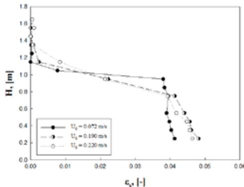
Fig. 3. Solid volume fraction of MWCNT agglomerates with axial height at  $U_0 = 0.072, 0.190,$  and  $0.220$  m/s.
