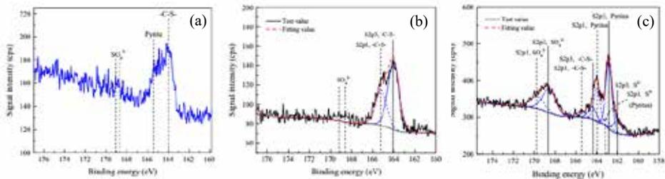
Fig.6 XPS Analysis result of raw coal, clean coal and gangue (a)raw coal (b)clean coal (c)gangue (Dong. L, 2015)
