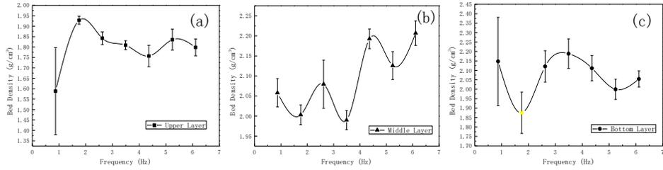
Fig.4 Bed density vs. gas pulsation frequency in pulsed fluidized bed (a)Upper layer; (b)Middle layer; (c)Bottom Layer;
