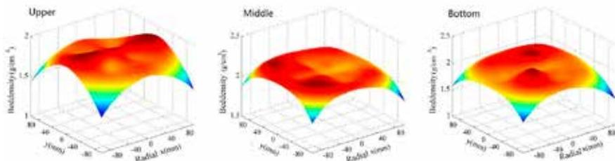
Fig.3 Contour of bed density at high-frequency region ( $f=5.24$  Hz)
