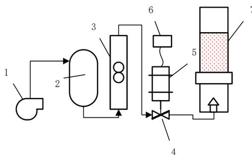
Fig. 1 Schematic of gas-vibro fluidized bed separation system: 1-Blower; 2-Buffer tank; 3-Flowmeter; 4-Butterfly; 5-Electric motor; 6-Inverter; 7- Fluidized bed.
