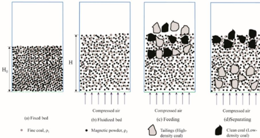
Fig. 2 Mechanism of the air dense medium separation (Y. Zhao et al., 2017)
