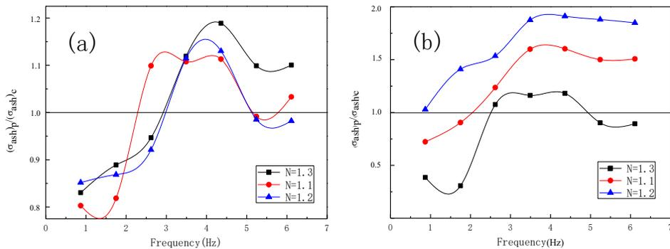
Fig. 5 Efficiency of pulsing gas flow on the separation of fine coal (a)-6+3 mm; (b) -3+1 mm
