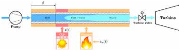
Fig. 2. Simple OTU boiler
