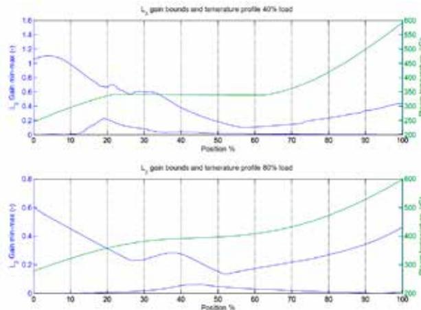
Fig. 3. Extremes of the control effort as a function of the position of solar share and the nominal temperature distribution of water-steam alongside the tube for subcritical (top) and supercritical (bottom) conditions
