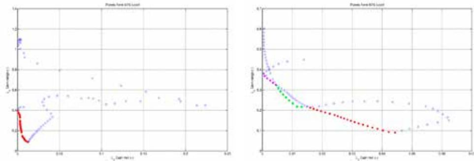
Fig. 5. Multi-objective plots of control efforts for subcritical (left) supercritical (right) conditions. The optimum in Pareto sense is colored.
