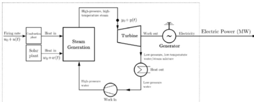
Fig. 1. Integrated solar-combustion thermal power plant
