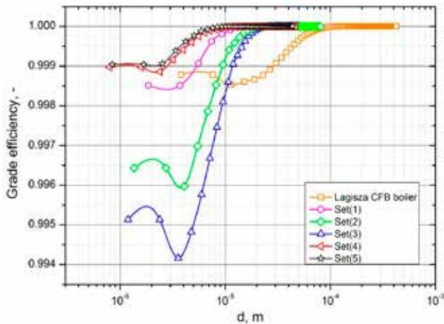
Fig. 5 Influence of the set of scaling relationships on the total grade efficiency curve
