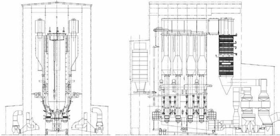
Fig. 1 Schematic diagram of the Lagisza 966MW<sub>th</sub> supercritical CFB boiler
