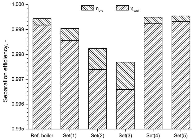
Fig. 3 Separation efficiency at the wall and in the inner vortex calculated for reference CFB boiler and scale cold models based on sets (1)-(5) (see Table 2)
