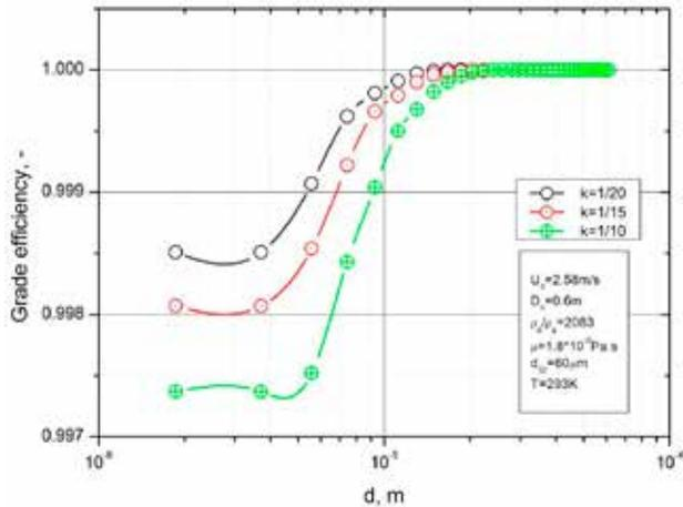
Fig. 4 Influence of a cold model scale factor 'k' on the total grade efficiency curve calculated for set(1) of scaling relationships
