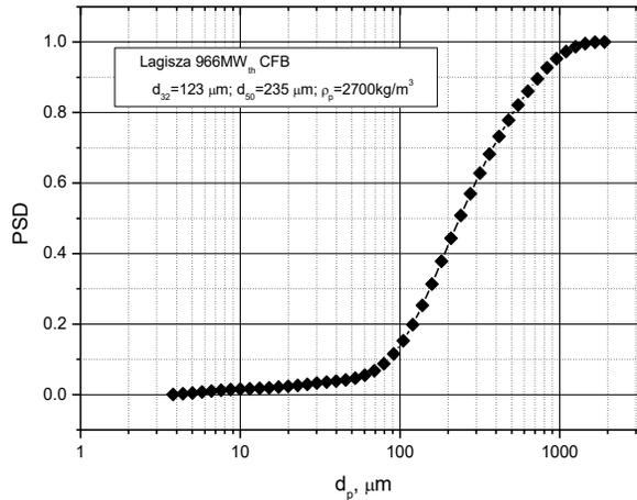
Fig. 2 PSD of inert material circulating in the Lagisza 966MW<sub>th</sub> CFB boiler
